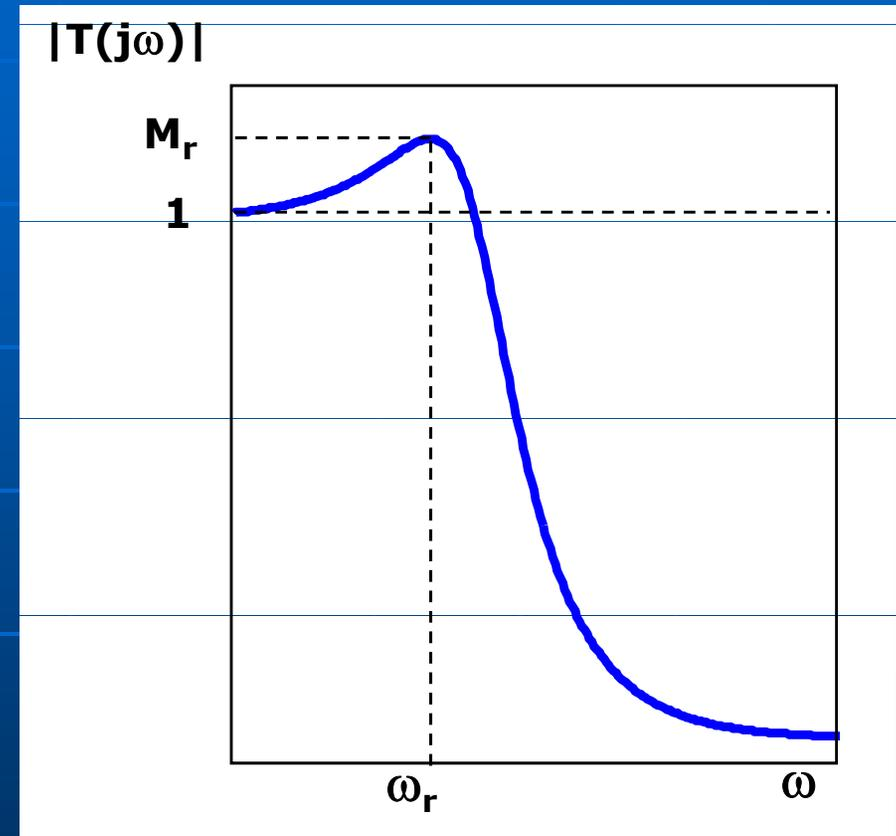
Note that resonant frequency is different than both the undamped and damped natural frequencies!
