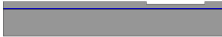
(c) 3 μm gap etching on the SOI wafer for the vertical axis accelerometer.
