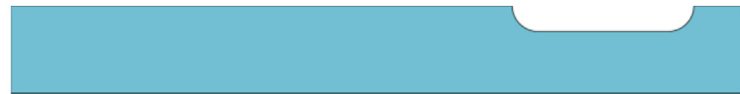
(a) Recess area formation over the glass wafer for the lateral axis accelerometers.
