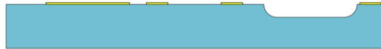
(b) Metallization to define the bottom electrode of the vertical axis accelerometer and contact metallization for lateral axis accelerometer.
