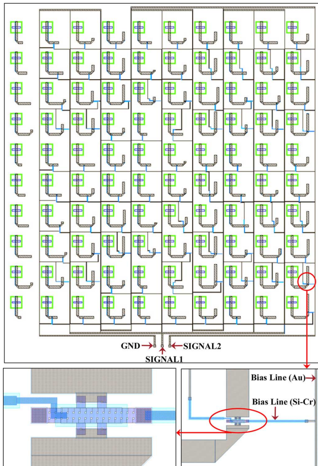
Fig. 6. Mask layout of a 10 \times 10 reflectarray with the RF MEMS switches.
