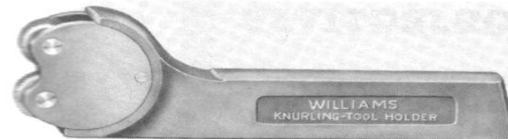
A knurling tool with one set of rolls in a self-centering head.
