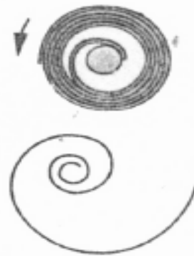
(h) Power or motor springs. Twist —exerts torque over many turns. Shown in, and removed from, retainer.
