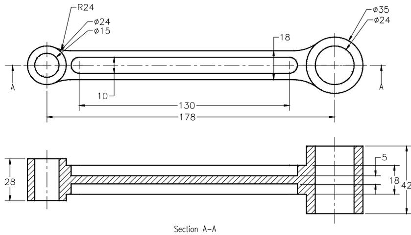
**Figure 4** Views and dimensions of the Articulated Rod
