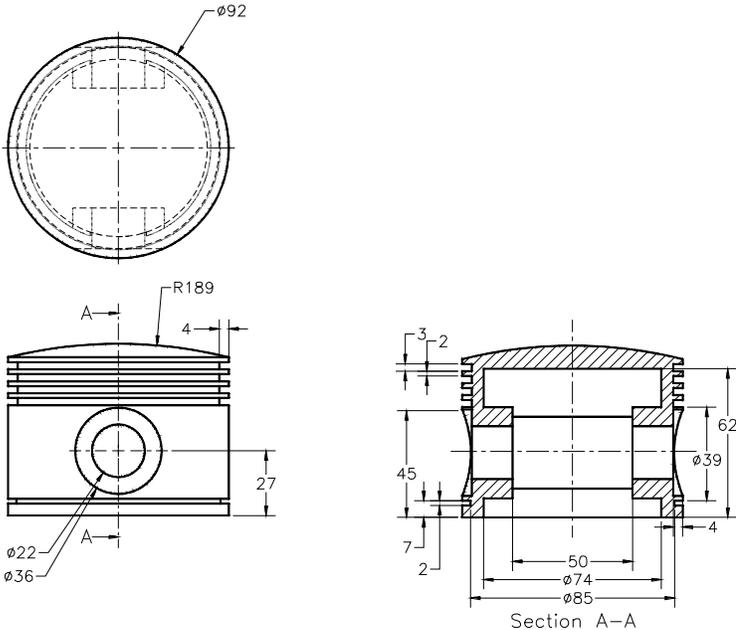
Figure 3 Views and dimensions of the Piston
