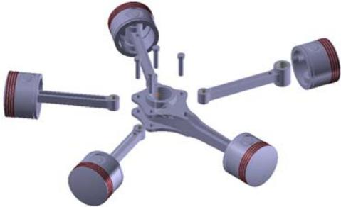
Figure 2 The exploded view of the assembly
