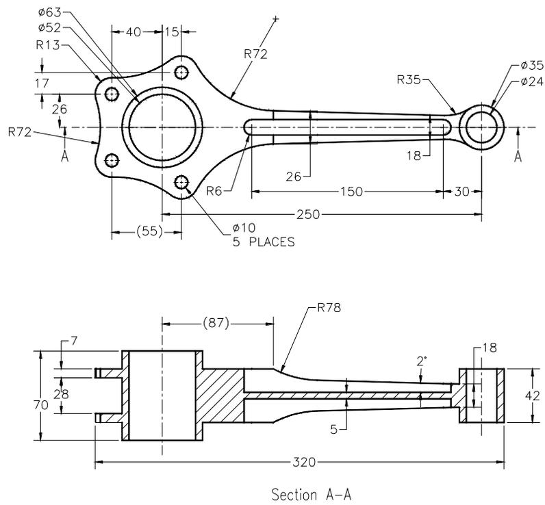
**Figure 5** Views and dimensions of the Master Rod
