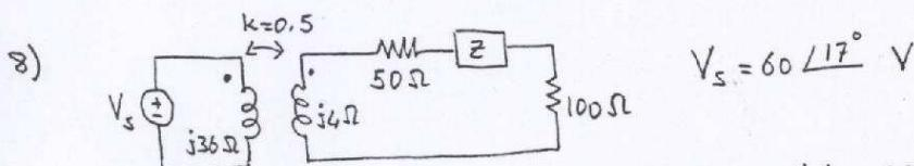
Determine Z so that the average power delivered to 100 ohm resistor is maximum. Also compute this power.
