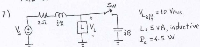
(a) SW is open: Find  $X$ ,  $\text{pf}_{\text{load}}$  and  $S_s$  given  $V_s_{\text{eff}} = 15 \text{ Vrms}$ .
