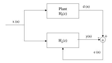
The unknown plant has the transfer function of the form:
