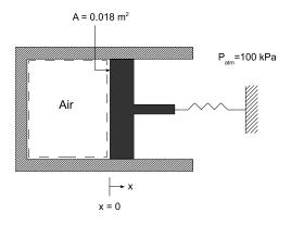
the cylinder wall. Determine the final pressure of the air, in kPa, and the work done by the air, in kJ.
