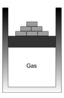
c. Consider the same system, but during the heat transfer let the weights be removed at such a rate that  $PV^{1.3}$  = constant describes the relation between pressure and volume during the process. Again the final volume is 0.1  $m^3$ . Calculate the work done.
