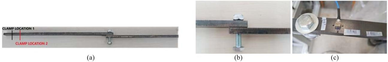
Figure 1: The experimental set-up of the beam measurements. (a) the beam structure with part A (left) attached to part B (right). The picture also shows the different clamping locations. (b) a close-up of the bolted joint unattached. (c) The beam in the setup with one of the PCB tri-axial sensors.
