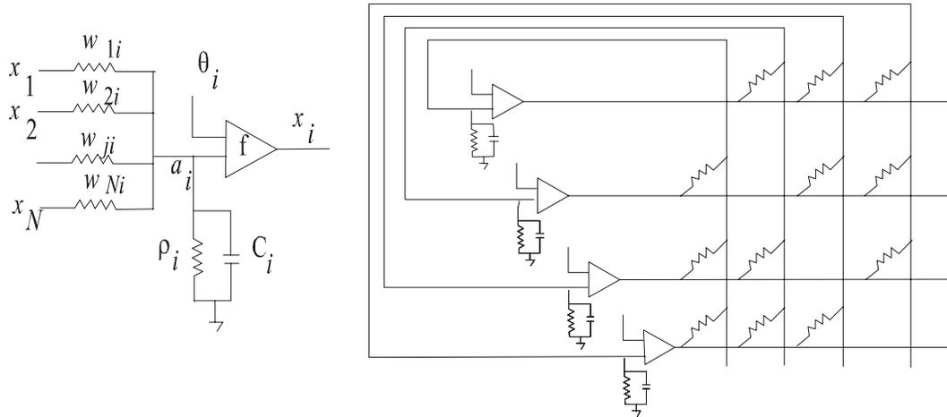
Figure 2.6 Hopfield Network made of electronic components
