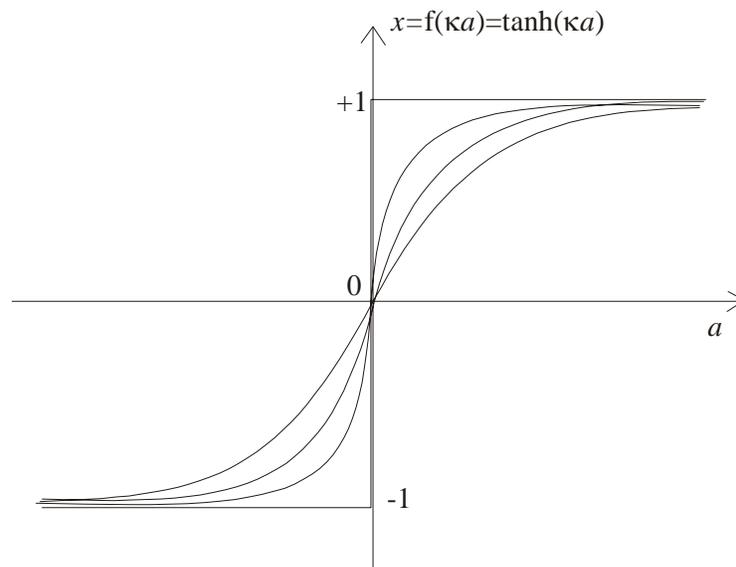
Figure 2.7 Output function used in Hopfield network
