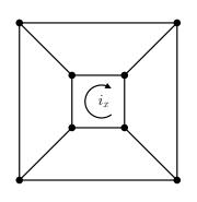
Consider the circuit  $\mathcal{N}$ . Note that " $e_x$  equals the sum of branch voltages associated to any path that connects the node  $n_x$  to the ground node." The dual of this statement for  $\mathcal{M}$  should read: " $i_x$  equals the sum of branch currents associated to any cut that connects the mesh  $m_x$  to the outer mesh." For example, take the path (in  $\mathcal{N}$ ) and its dual cut (in  $\mathcal{M}$ ) shown below. For this particular path-cut pair our dual statements yield
