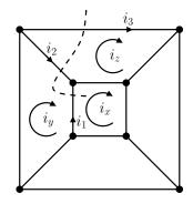
The fact that  $i_x$  is independent of the cut, provided that the cut connects  $m_x$  to the outer mesh, gives  $i_x$  at once a physical character. Namely, the mesh current  $i_x$  is the (well-defined) current circulating in the ring (or "donut") where the inner circle of the ring is contained in the mesh  $m_x$  while the outer circle of
