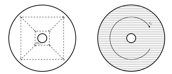
Thanks to this simple observation the question on measuring  $i_x$  we asked earlier can now be rephrased: What instrument does one use to measure the current circulating within a "donut"? The answer is clamp-on ammeter. The below figure shows the dual measurements of  $e_x$  and  $i_x$  by a voltmeter and a clamp-on ammeter, respectively. This allows us to conclude that mesh currents are as measurable and hence as real as node voltages.
