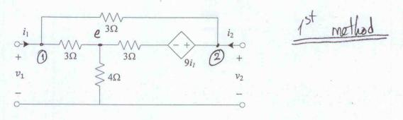
$$\frac{e - 2i}{3} + \frac{e + 9i_1 - 2i_2}{3} + \frac{e}{4} = 0 \Rightarrow e = \frac{4}{11} 2i_1 + \frac{4}{11} 2i_2 - \frac{36}{11}i_1$$
