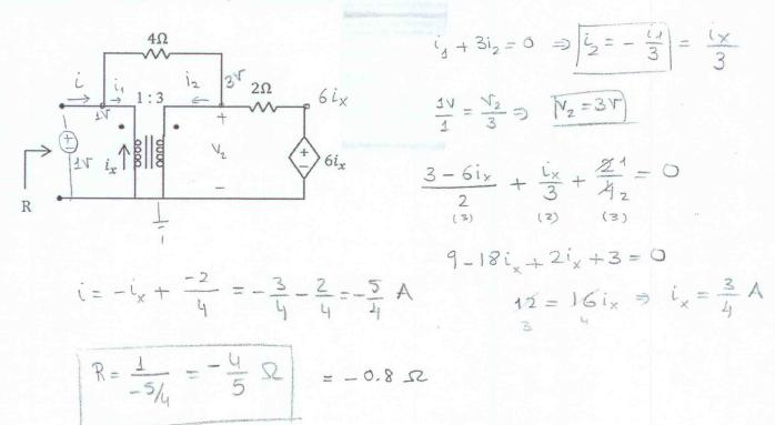
**Question 2 (14 pts)** The one-port circuit N in the figure below is made up of passive LTI resistors and constant independent sources. The Thevenin resistance of N is denoted by  $R_{TH}$ . R is a passive LTI resistor. The power delivered to R is denoted by P.
