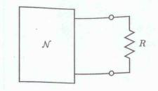
(7) a) It is observed that for two different values of R, R<sub>1</sub> and R<sub>2</sub>, P has the same value. Show that  $\sqrt{R_1R_2} = R_{TH}$ .
