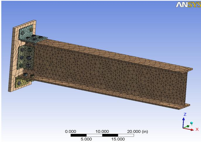
**Figure 2.** A sample finite element mesh for the top and seat angle with double web angles connection
