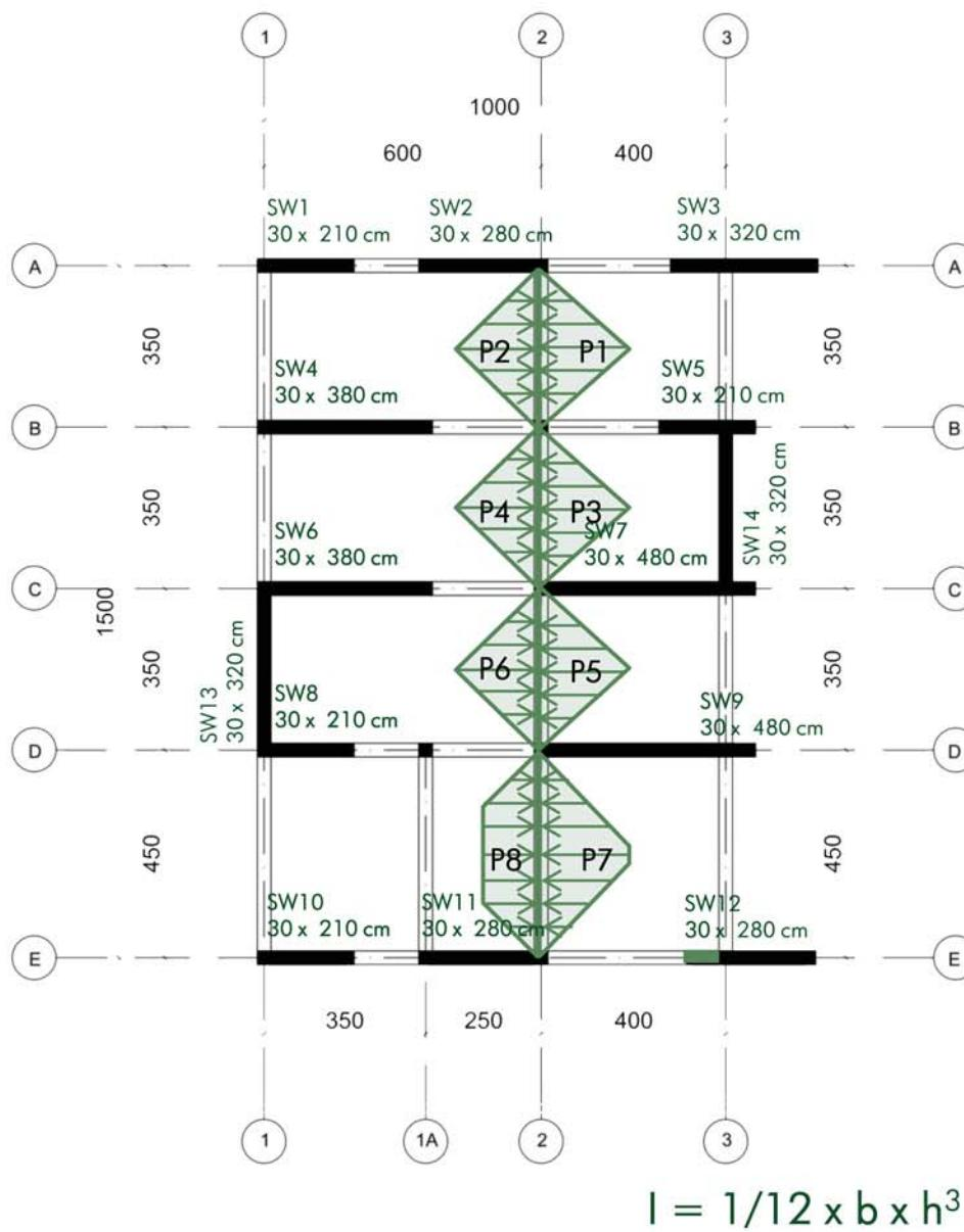
$$I_{beam} = 1/12 \times (0,30) \times (0,48)^3 = 2,76 \times 10^{-3} \text{ m}^4$$
