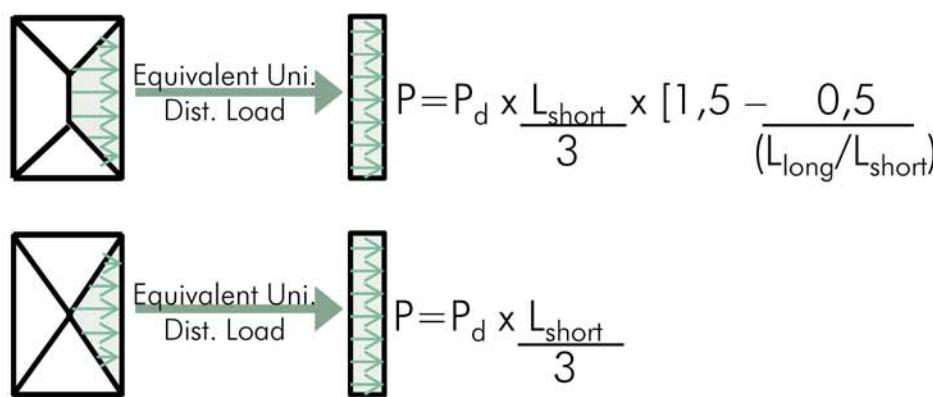
$$P_d = (\text{Dead Load} \times \text{Load Factor}) + (\text{Live Load} \times \text{Load Factor})$$
