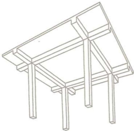
Selected slab type is solid slab with beams. Since,  $l_l / l_s \leq 2$ . Then two way solid slab system should be utilised.
