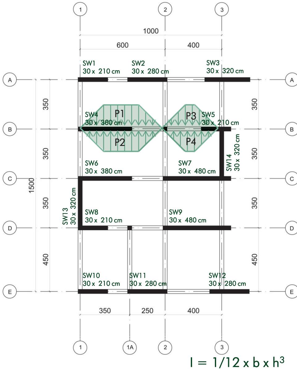
$$I_{beam} = 1/12 \times (0,30) \times (0,48)^3 = 2,76 \times 10^{-3} \text{ m}^4$$
