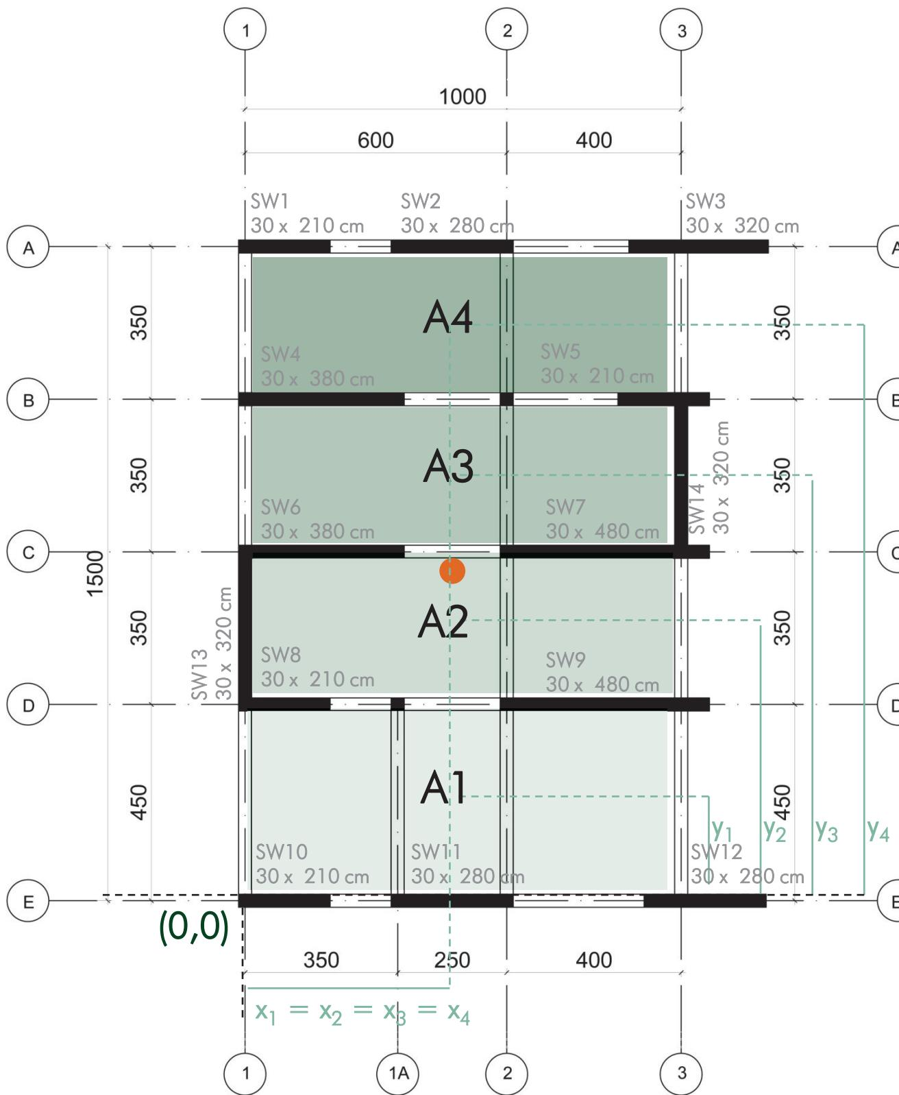
Since the plan has a simple geometry, it can be easily understood that geometric center is (5, 7.5). However, the detailed calculations are as follows:
