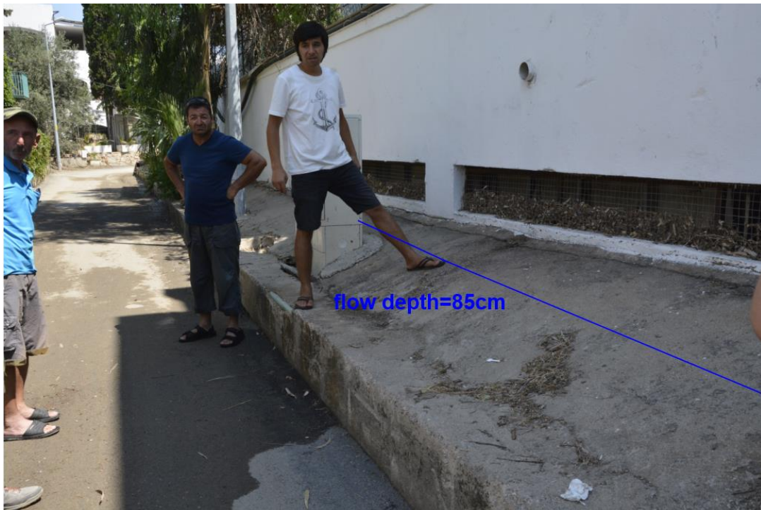
Figure 4.4: Observer showing the flow depth by his foot (37.031412N 27.406703E)
