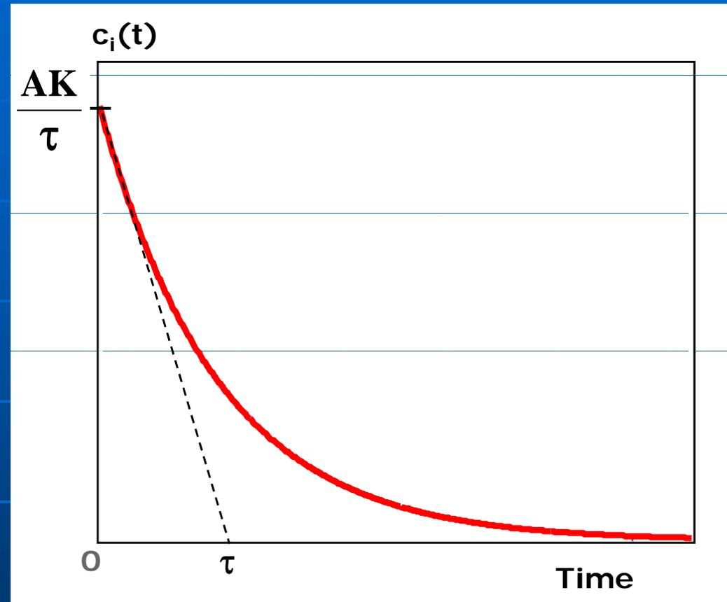
It is observed that the initial slope intersects the time axis at  $\tau$  – **How can this be useful ?**
