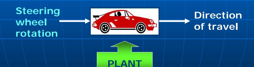
**Process:** is an operation to be controlled.
