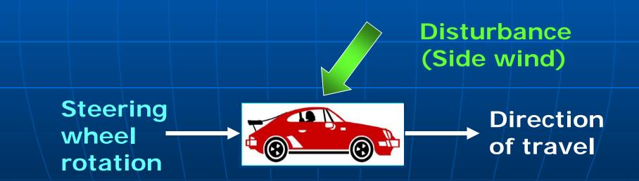
**Disturbance input**: is an unwanted input that tends to adversely affect the value of the output of a system.
