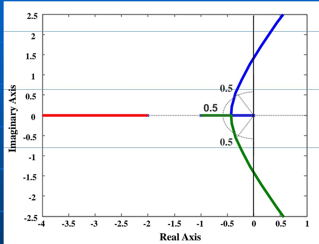
to get the constant undamped natural frequency and damping ratio lines.
