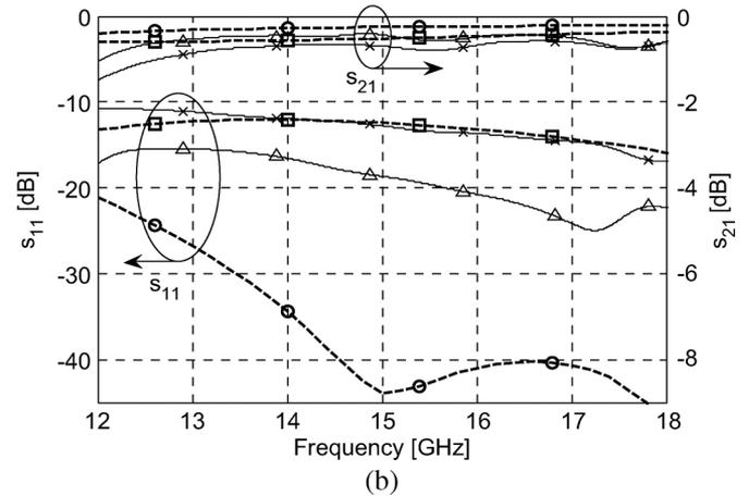
Fig. 4. Measured and simulated  $S$ -parameters of the MEMS CRLH unit cell.
