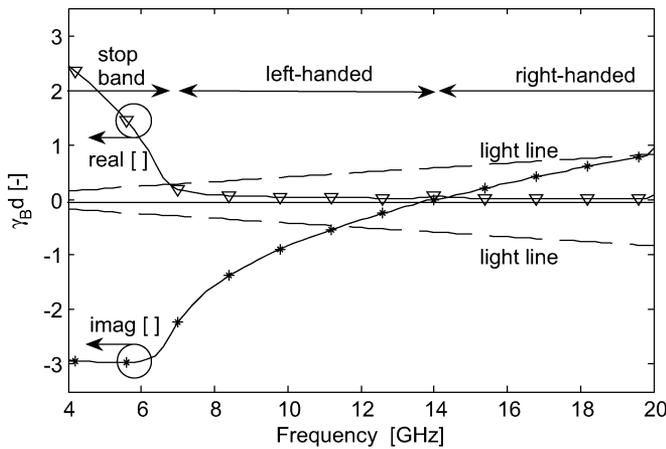
Fig. 3. Simulated Bloch-Floquet propagation constant of the MEMS CRLH unit cell without actuation (using Ansoft HFSS).
