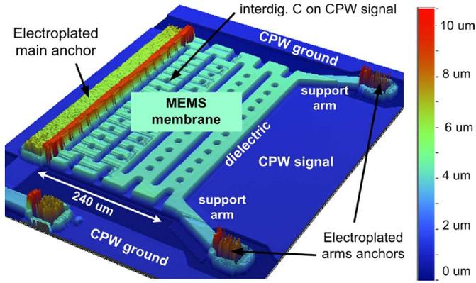
Fig. 2. Measured profile of the non-actuated fabricated MEMS. The membrane is suspended over the targeted air gap of  $2\ \mu\text{m}$  and exhibits good planarity.
