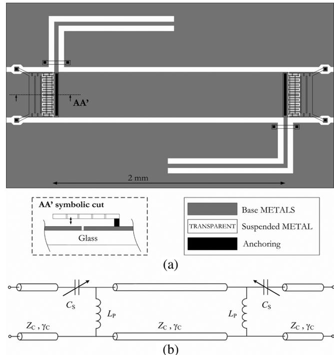
Fig. 1. (a) Layout of the CRLH unit cell and cross-sectional view of the MEMS capacitor. For clarity, the two first metal layers are shown as one (base metals) and dielectric and sacrificial layers are omitted. (b) Corresponding CRLH unit cell circuit model (without parasitic elements).
