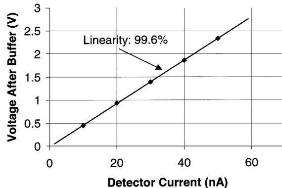
Fig. 7. Measurement results of the fabricated CMI unit cell, verifying its functionality and linearity.
