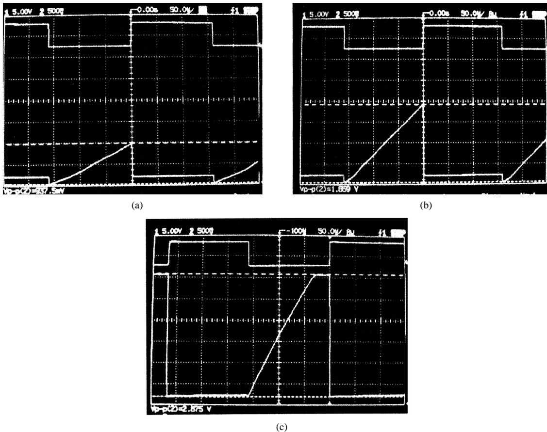
Fig. 6. Measurement results of the CMI unit cell with simple source follower buffers for different detector current values: (a) 20 nA, (b) 40 nA, and (c) 70 nA, while the integration time is fixed at 120  $\mu$ s.
