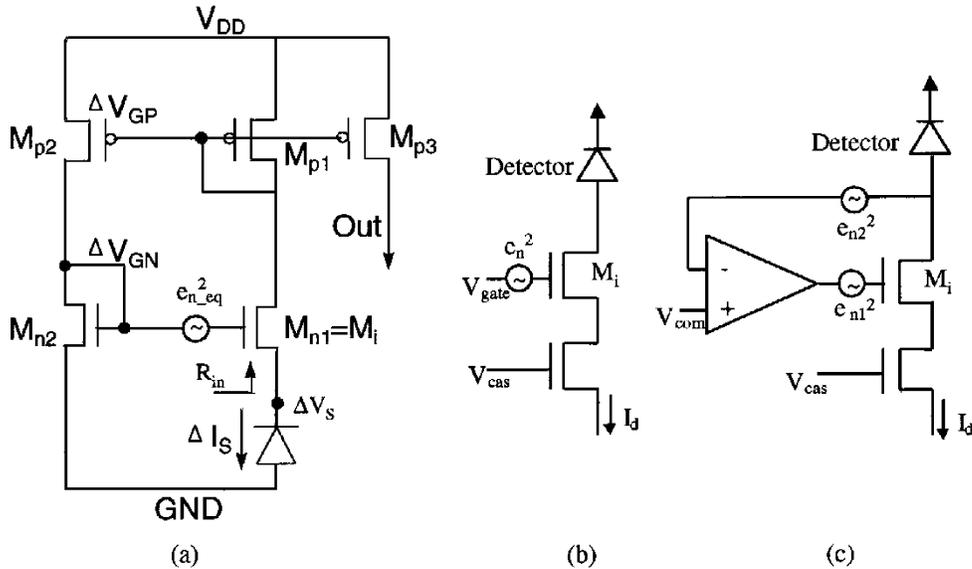
Fig. 2. Simplified schematic view of various preamplifier structures used for analytical calculations and noise comparisons: (a) CMI, (b) DI, and (c) BDI structures.
