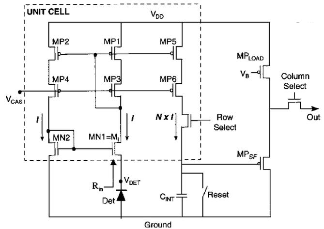
Fig. 1. Schematic view of the CMI preamplifier circuit, including the unit cell and off-pixel components.
