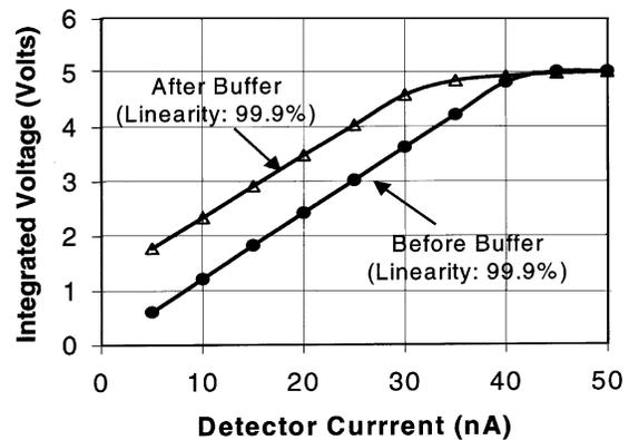
Fig. 4. Integrated voltage values obtained for different detector currents both before and after the source follower buffer, while the integration time is fixed at 120  $\mu$ s. These results show that the CMI circuit provides linearity better than 99% for an output voltage swing between 0 and 4.5 V before and after the source follower buffer.
