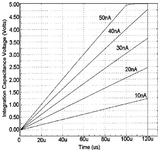
Fig. 3. Simulation results of the CMI circuit. The waveform shows the integration curves for various current values, verifying the high linearity and high output voltage swing. Here, the integration capacitance is chosen as 1 pF to show the dynamic range.
