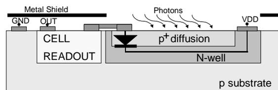
Fig. 1: The structure of CMOS visible image sensor. p-n junction diode is implemented with p+ diffusion and n-well.
