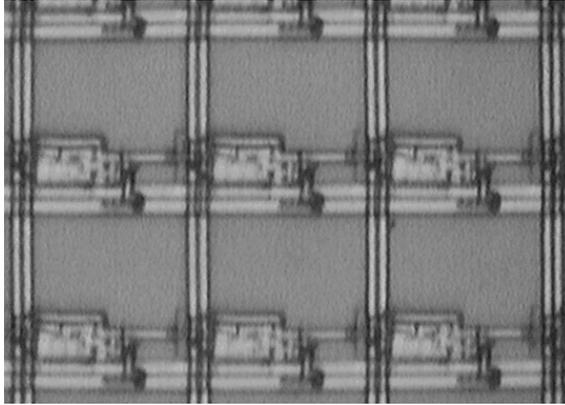
Fig. 9: The close up microphotograph of the fabricated 16x16 test array showing few pixels. The bottom left part of the unit cells are the CMI readout transistors shielded by the second metal layer.
