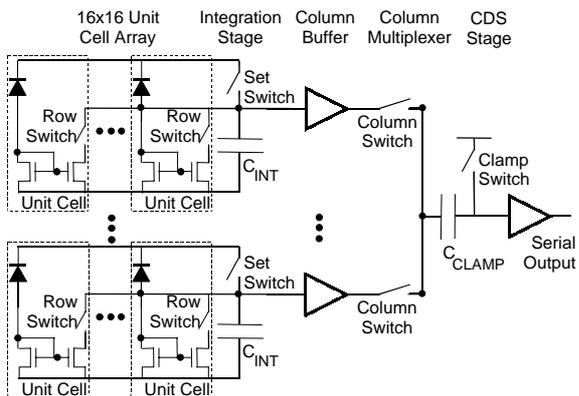
Fig. 4: Overall datapath for the focal plane array. The integration capacitor voltage is buffered and multiplexed by the column select switches. The multiplexed data is processed by the correlated double sampling (CDS) circuit and a single serial output is generated.
