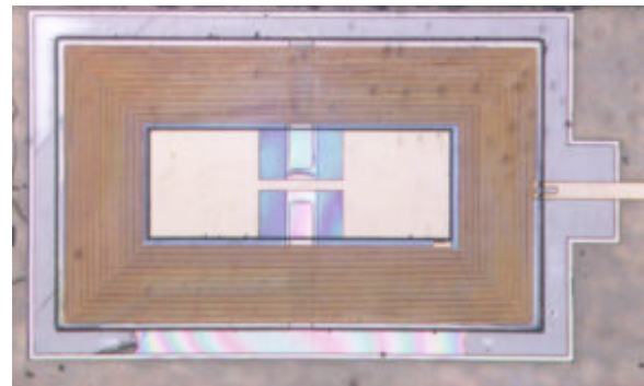
Fig. 5: Photograph of a fabricated sensor seen through the glass substrate. This device measures 2.6\text{mm}\times 1.6\text{mm} and houses 24 turns of gold-electroplated coil. The capacitive plate separated into two parts to increase the dynamic range.
