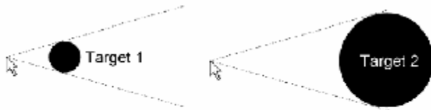
Figure 2.3: Scale invariance of Fitts' law: the two targets illustrated require the same time to select, because the ratio of A/W is the same in both cases.
