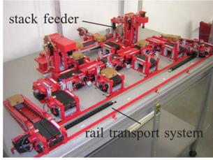
Fig. 9. Fischertechnik manufacturing system model.
