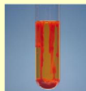
Iron(III) chloride, FeCl_3 (Here forming as the solid at the bottom of the test tube) Orange-brown color Density 2.90 \text{ g cm}^{-3} Melts at 306^\circ\text{C}
