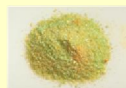
Iron(II) chloride, FeCl_2 Greenish-yellow color Density 3.16 \text{ g cm}^{-3} Melts at 670^\circ\text{C}
