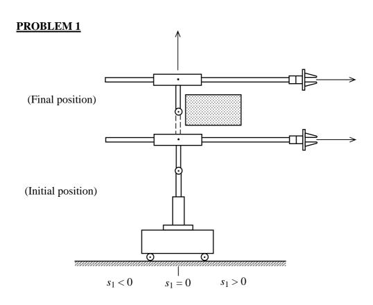
As one of the tasks to be conducted, two successive positions of the robot in Problem 7 of Set 2 are shown in the figure. The shaded rectangle represents an obstacle that must be avoided by the robot as it conducts this task.
