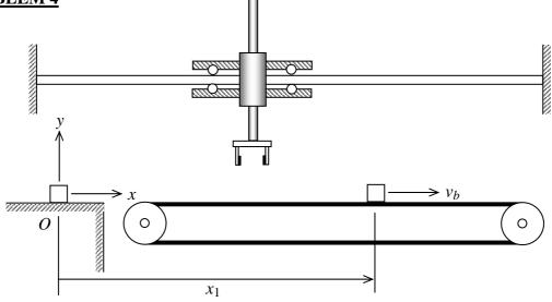
The figure shows a *gantry robot* having prismatic joints in the x and y directions. It is to be used for a task of picking up an object from a conveyor belt, carrying and dropping it to the origin O of the xy-frame, and doing the same for the next object.
