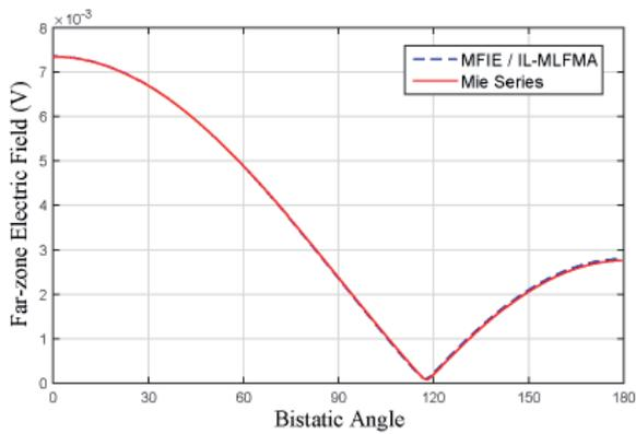
**Figure 3. The solution of the problem SOLBOX-03 using a broadband implementation of MLFMA, compared to the Mie-series results.**
