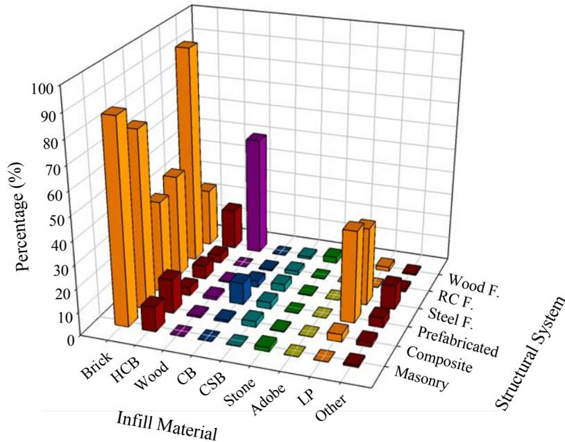
**Figure 5.** Percentages of infill wall material with respect to structural system
