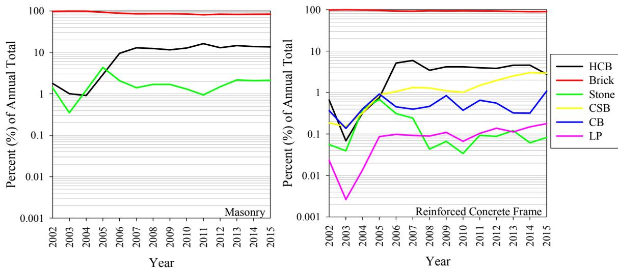
**Figure 6.** Annual variation of infill wall material of masonry and RC frame buildings
