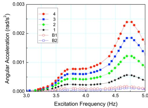
**Figure 5 – Acceleration-frequency curves for torsional responses of all floors.**
