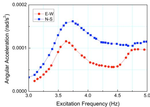
**Figure 6 – Acceleration-frequency curves for rocking response of the building.**
