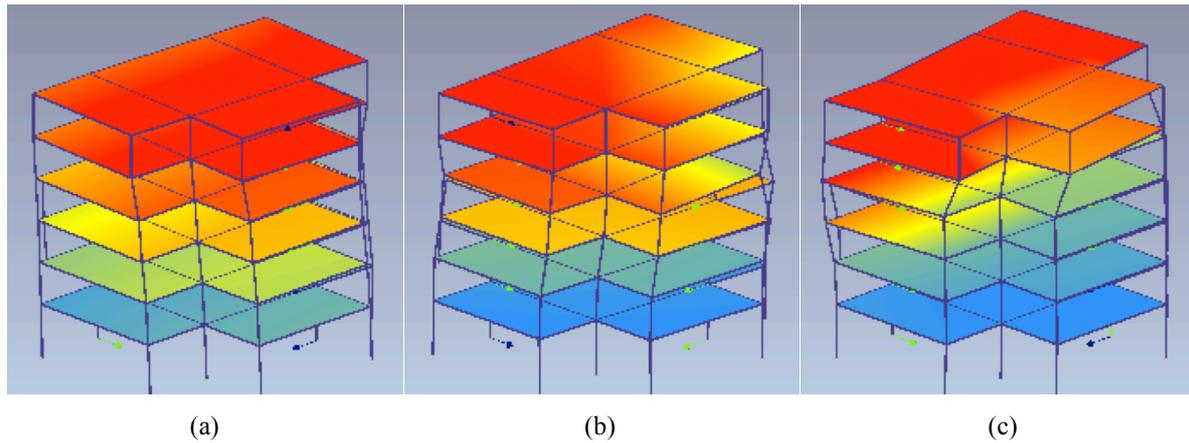
**Figure 6.** Mode shapes: (a) E-W translational, (b) N-S translational, (c) torsional.
