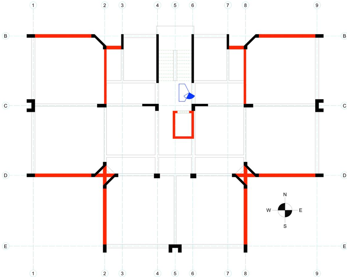
**Figure 2.** Fourth floor plan; Vibration generator location.
