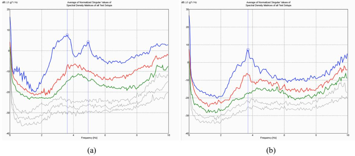
**Figure 4.** Singular values of the power spectral density matrices of the ambient responses: (a) E-W and (b) N-S setups.
