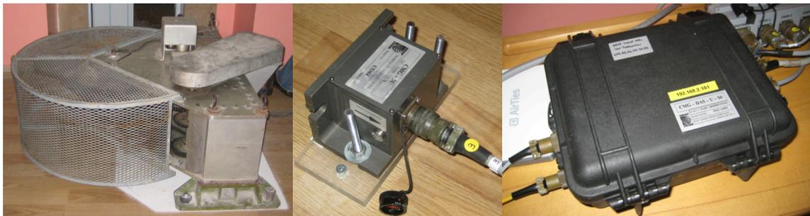
**Figure 3.** (a) Vibration generator, (b) accelerometer #3, (c) data acquisition system.
