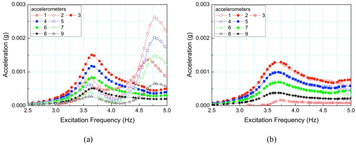
**Figure 5.** Acceleration-frequency response curves for (a) E-W and (b) N-S excitations.
