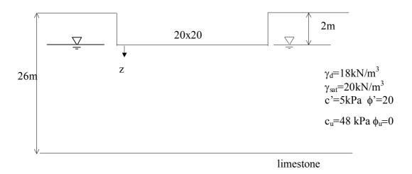
Skempton expression for  $\phi_u$ =0 is :  $q_f$  =  $c_uN_c$  +  $\gamma_{sat}$  D (total stress analysis)  $q_{nf}$  =  $c_uN_c$
