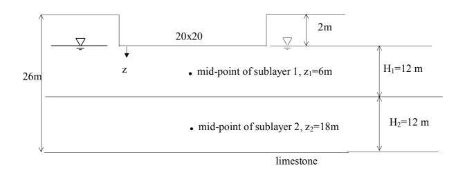
• Vertical Stress due to q<sub>net</sub> should be determined at the mid-point of each sublayer
