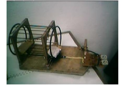
Saddle type. 30 cm diameter. 3 turns each side. Tuned to 6.4 MHz.
