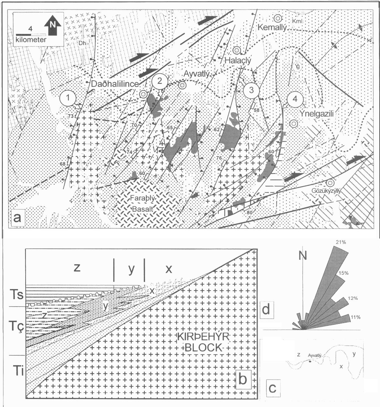
**Fig. 8:** a) Geological map of the central part of the Çankırı Basin. b) simplified map of the facies belts of the Çandır Formation, c) schematic illustration of the interpreted cross-section of facies belts of the Çandır Formation, d) length weighted rose diagram of the faults that are displacing the granitic basement and the Çandır Formation, percentages indicate the length frequency of the faults (see Figure 5 for the explanation of the symbols).
