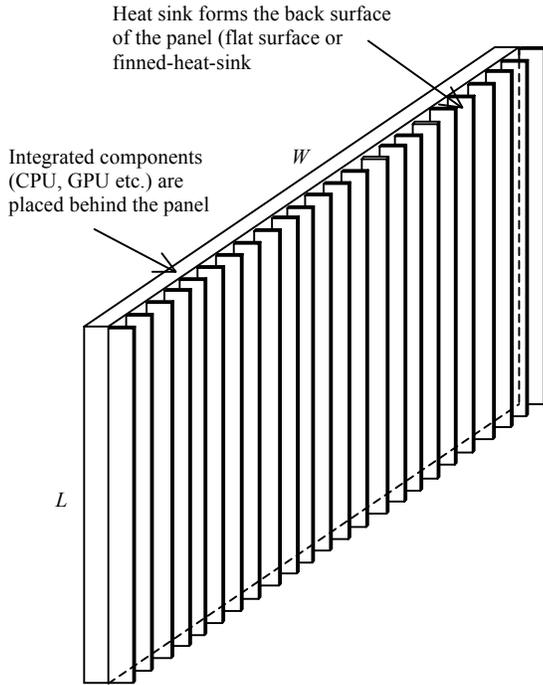
Fig. 2. Plate finned vertical heat sink geometry.
