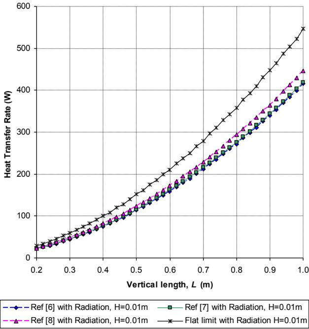
Fig. 7. Passive heat transfer rates (natural convection and radiative transfer) for the fin height,  $H=0.01$  m.
