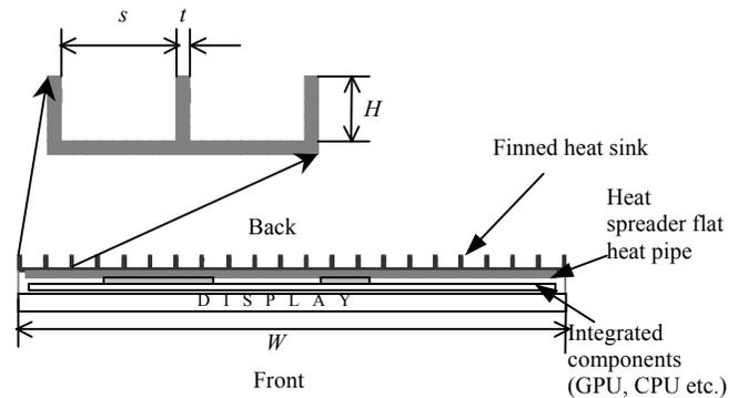
**Fig. 1. Top view of the passive cooling heat sink assembly. Heat spreader flat heat pipe is in contact with the integrated components. Plate finned heat sink is attached to the heat spreader. Heat is dissipated from the heat sink with natural convection and radiation.**
