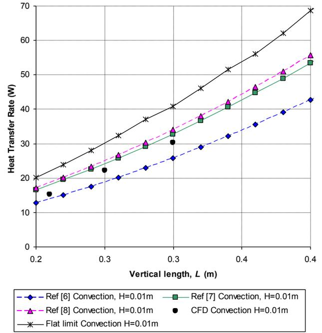
Fig. 6. Natural convection heat transfer rates without radiative transfer for the fin height,  $H=0.01$  m, comparison of 3 data points obtained from CFD simulations with the results of correlations.
