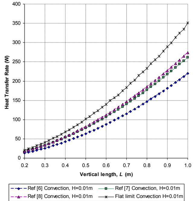
Fig. 4. Natural convection heat transfer rates without radiative transfer for the fin height,  $H=0.01$  m.
