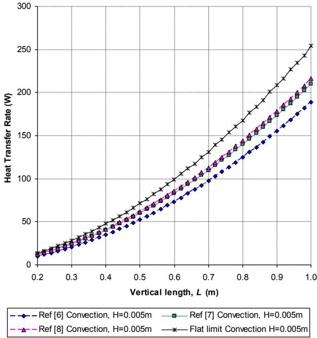
Fig. 5. Natural convection heat transfer rates without radiative transfer for the fin height,  $H=0.005$  m.
