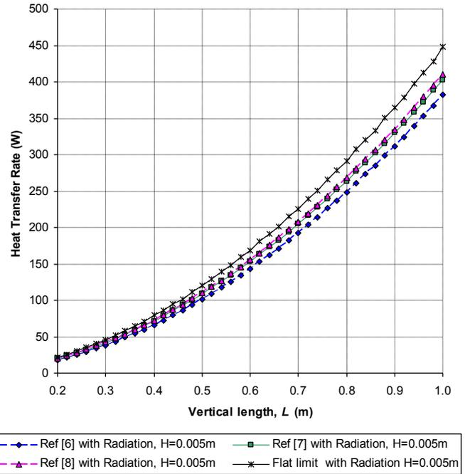
Fig. 8. Passive heat transfer rates (natural convection and radiative transfer) for the fin height,  $H=0.005$  m.
