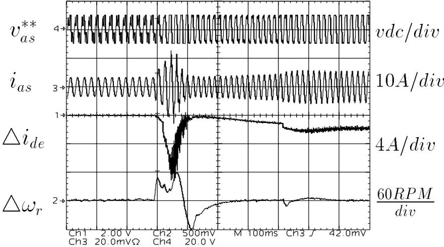
Figure 5.40: DPWM2 modulation signal, phase current, d axis current error, and speed error oscillograms.
