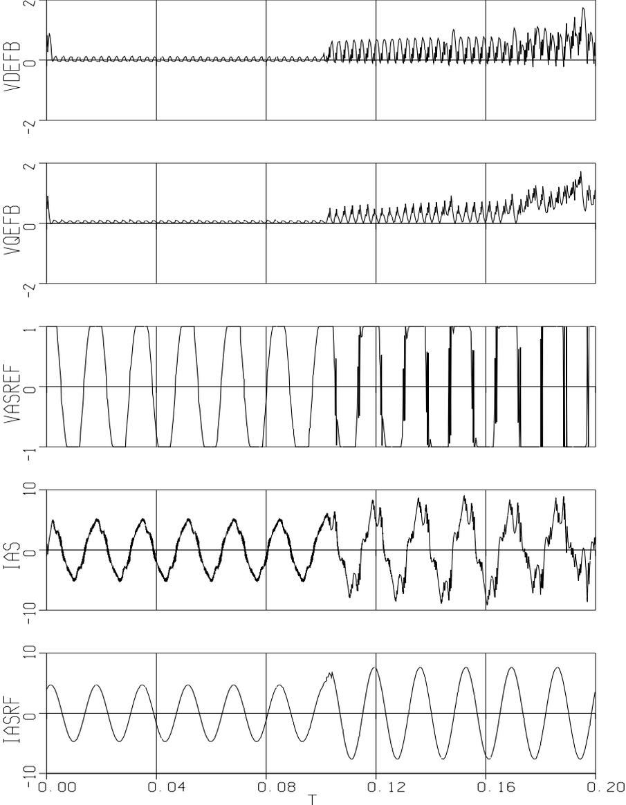
Figure 5.44: SFCR based system simulation waveforms in the overmodulation range. Traces (bottom to top): reference and actual phase currents, DPWM1 modulation wave, q and d axis PI controller outputs. At  $t = 0.1s$ ,  $M_i$  is increased from 0.933 to 0.975.
