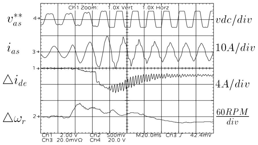
Figure 5.43: SVPWM modulation signal, phase current, d axis current error, and speed error oscillograms.
