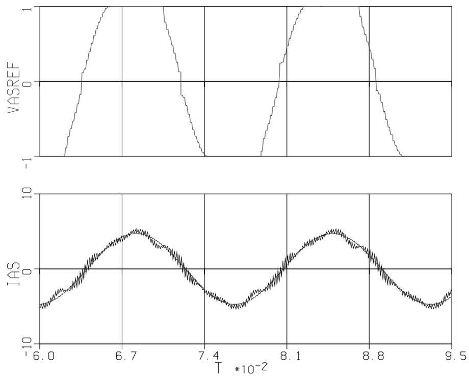
Figure 5.46: Zooming into the phase current and modulation wave at  $M_i = 0.933$ . Traces (bottom to top): reference and actual phase currents, and DPWM1 modulation wave.
