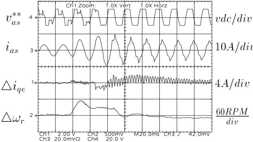
Figure 5.30: DPWM0 modulation signal, phase current, q axis current error, and speed error oscillograms: zoomed view of the first few cycles.
