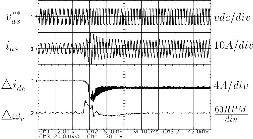
Figure 5.31: DPWM0 modulation signal, phase current, d axis current error, and speed error oscillograms.
