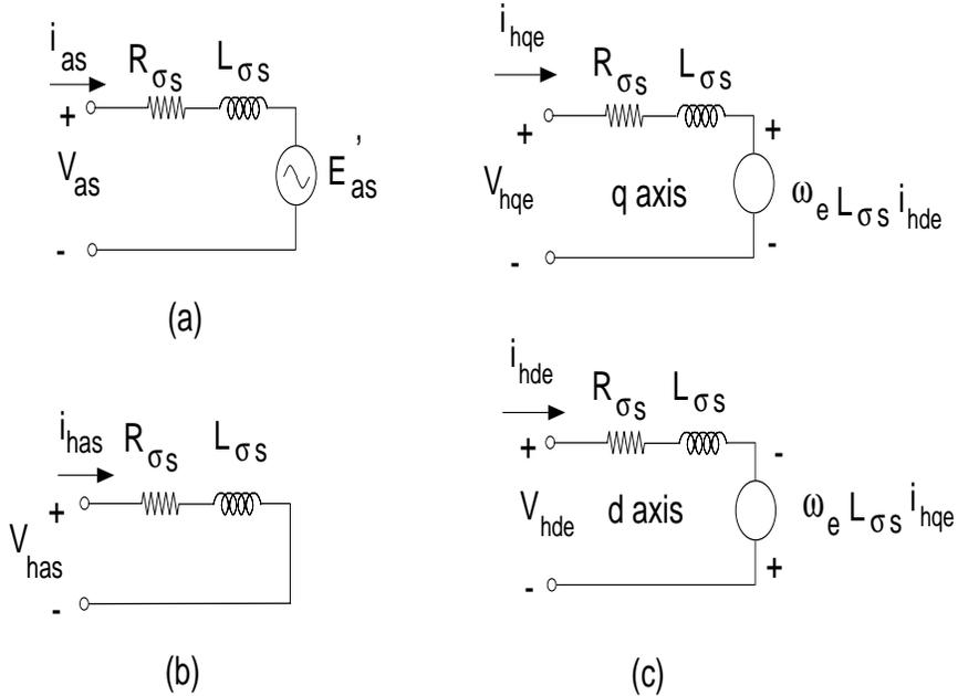
Figure 5.47: Three phase AC induction motor transient and harmonic equivalent circuits; (a): Per phase fundamental component transient model, (b): Per phase harmonic model, (c): Harmonic model in the synchronous frame.
