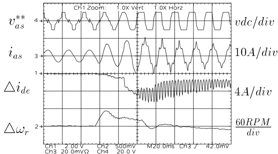
Figure 5.36: DPWM1 modulation signal, phase current, d axis current error, and speed error oscillograms.
