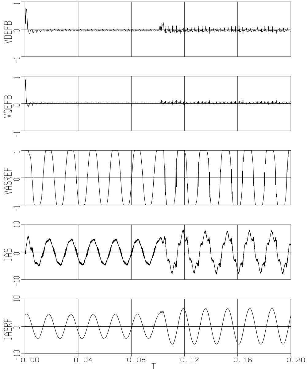
Figure 5.49: Harmonic feedback reduced, SFCR based drive simulation waveforms in the overmodulation range. Traces (bottom to top): reference phase current, actual phase current, modulation wave, q and d axis PI controller outputs. At  $t = 0.1s$ , the modulation index is increased from  $M_i = 0.933$  to  $M_i = 0.965$ .
