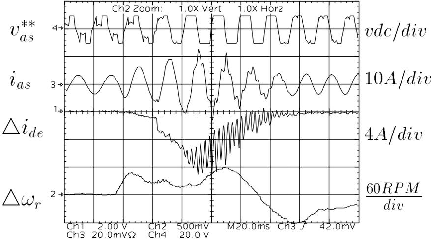
Figure 5.39: DPWM2 modulation signal, phase current, d axis current error, and speed error oscillograms.
