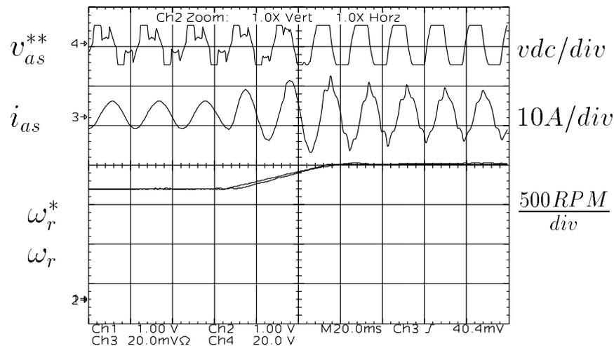
Figure 5.33: DPWM0 modulation signal, phase current, speed and speed reference oscillograms.
