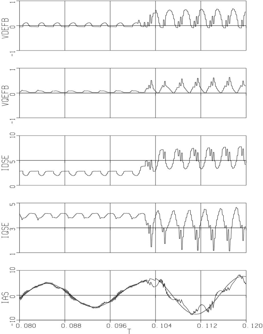
Figure 5.45: Detailed view of the system characteristic waveforms in the over-modulation range. Traces (bottom to top): reference and actual phase currents, discretized q and d axis currents, q and d axis PI controller outputs.
