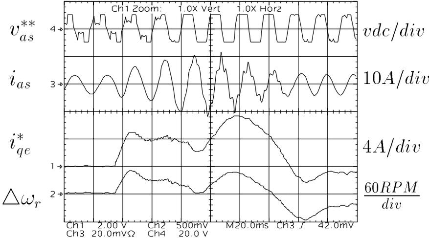
Figure 5.37: DPWM2 modulation signal, phase current, q axis current reference, and speed error oscillograms.
