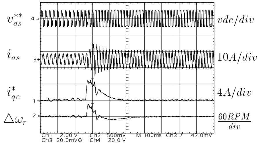
Figure 5.27: DPWM0 modulation signal, phase current, q axis current reference, and speed error oscillograms.
