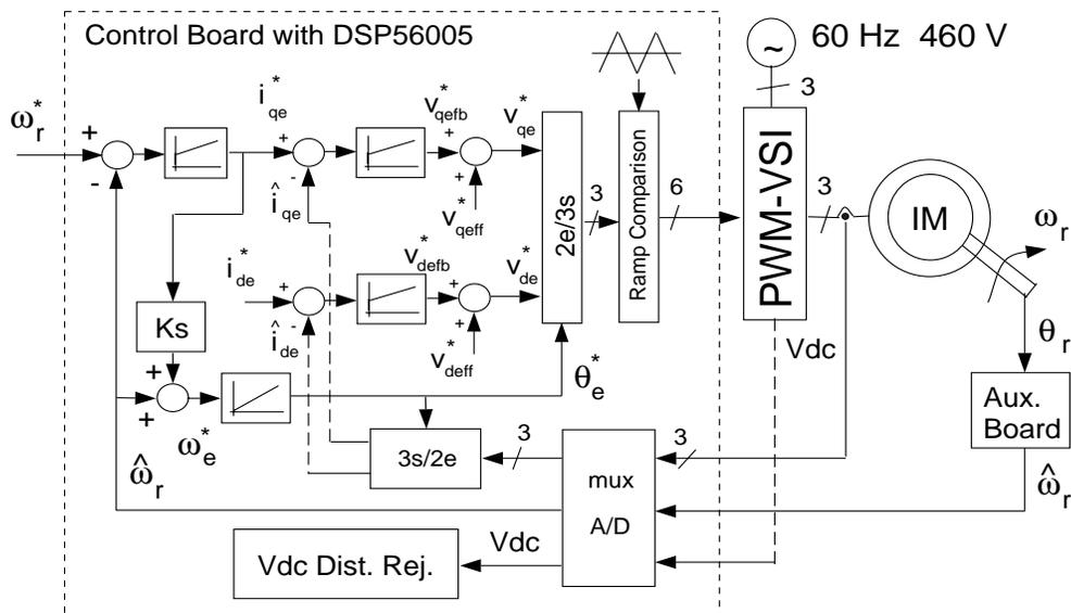
Figure 5.26: The experimental RFO-IFOC drive control diagram.
