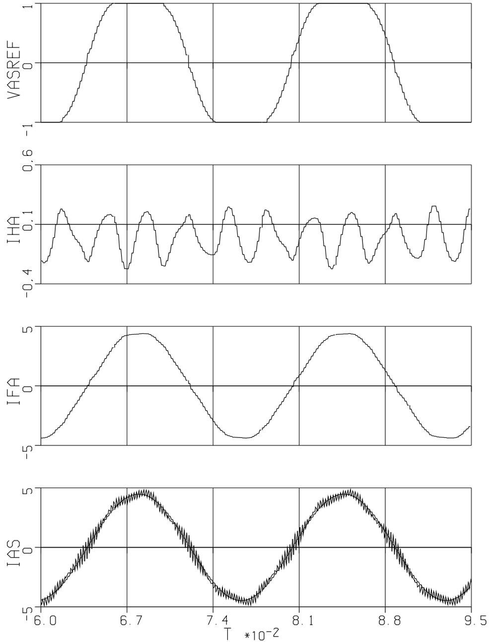
Figure 5.51: Zoomed view of the phase current and modulation wave at  $M_i = 0.933$ . Traces (bottom to top): reference and actual phase currents, estimated fundamental component and harmonic currents, and DPWM1 modulation wave.
