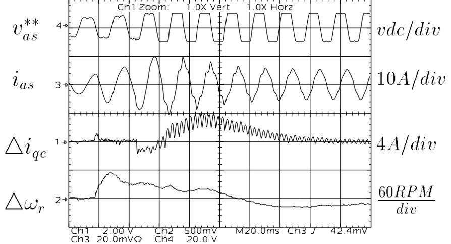
Figure 5.42: SVPWM modulation signal, phase current, q axis current error, and speed error oscillograms.
