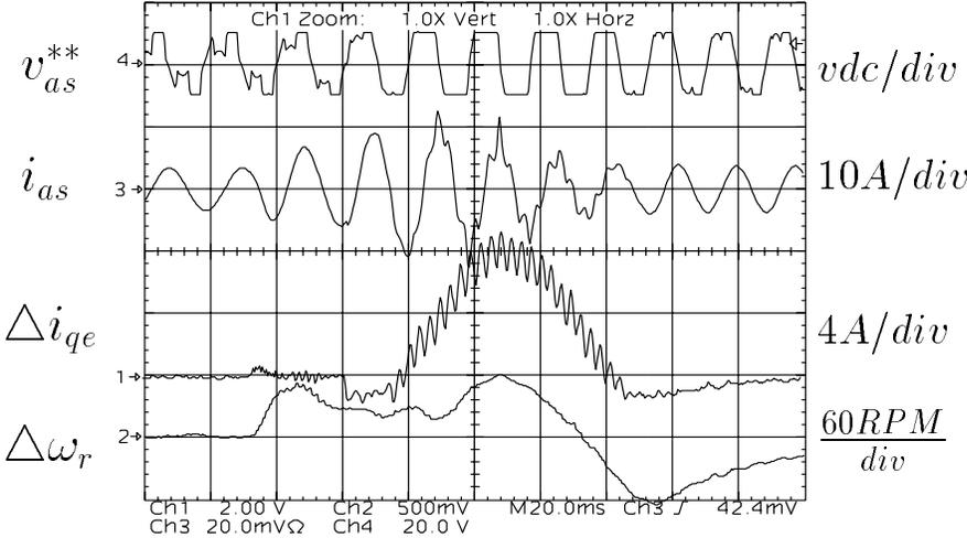
Figure 5.38: DPWM2 modulation signal, phase current, q axis current error, and speed error oscillograms.
