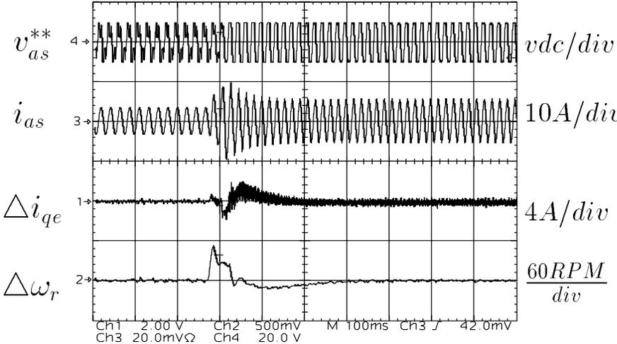
Figure 5.29: DPWM0 modulation signal, phase current, q axis current error, and speed error oscillograms.
