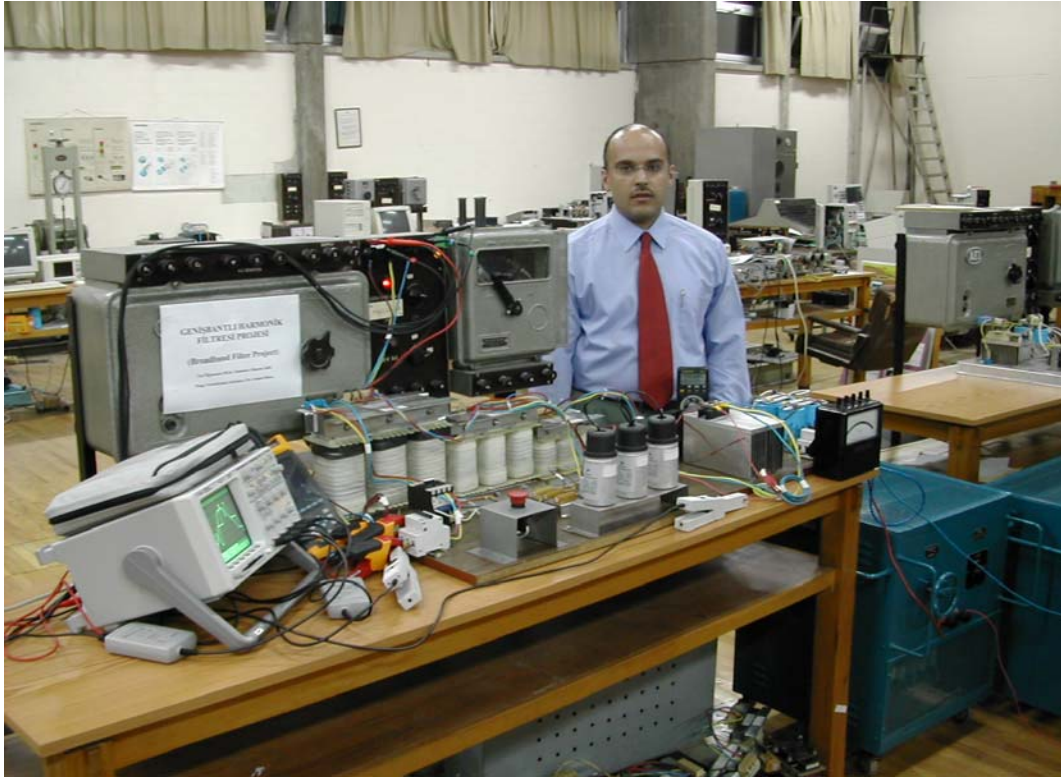
Fig. 5.40 Photograph of the overall laboratory test system involving 5.5 kW IBF.
