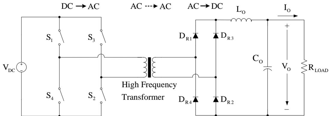
Figure 1.4 The full-bridge DC/DC converter basic circuit configuration.
