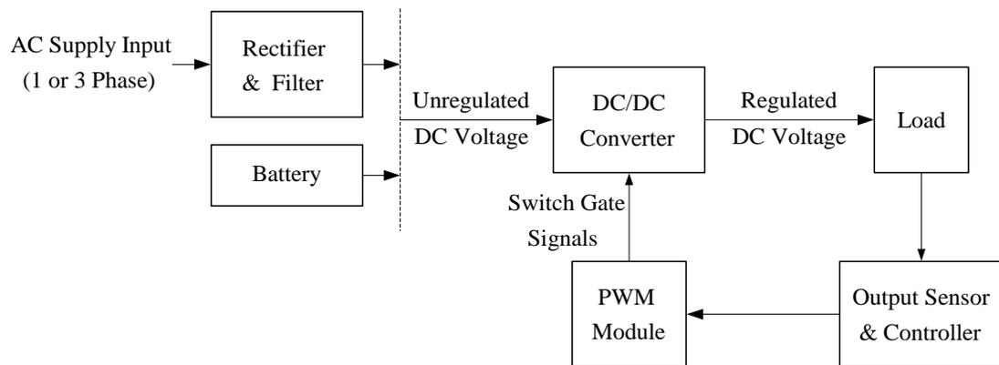
Figure 1.1 Generalized block diagram of an SMPS system.
