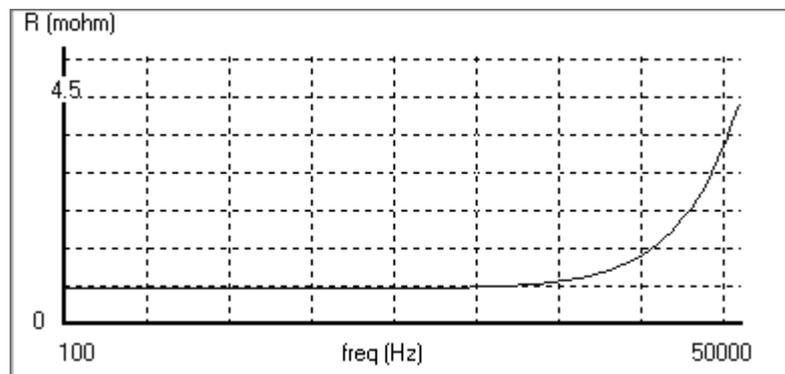
Figure 4.10 The secondary winding resistance obtained by FEA.
