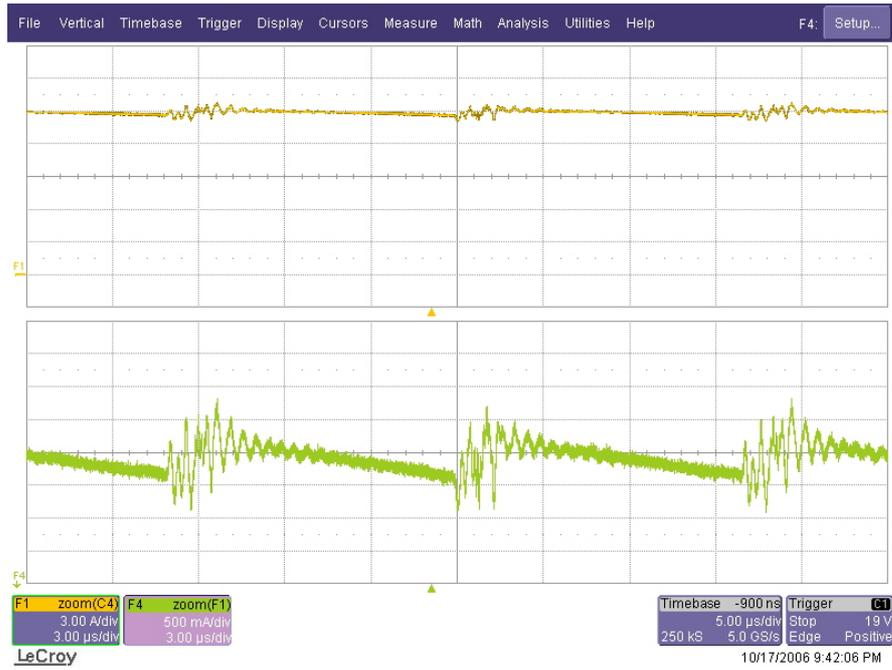
Figure 6.25 Load current waveform (top) and its vertically zoomed version (bottom) at 15% load (scales: 3 A/div, 500 mA/div, 3 μs/div).
