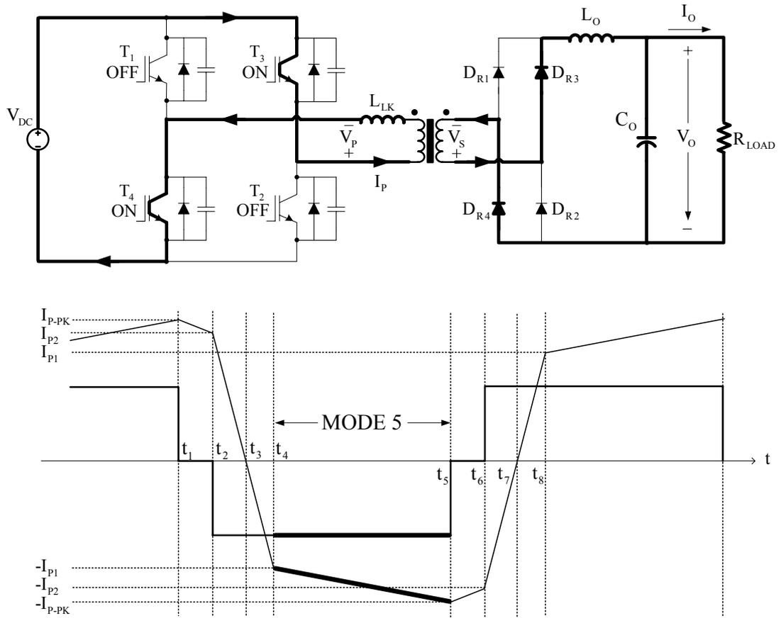
Figure 3.16 The circuit diagram and primary voltage and current waveforms of the FB-PS-ZVS DC/DC converter in mode 5.
