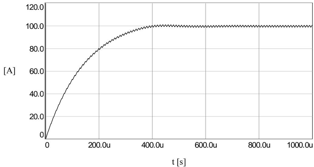
Figure 5.28 Step response performance of the output current controller.
