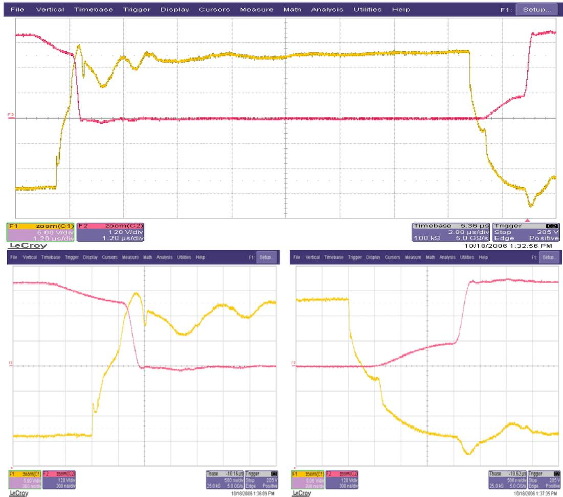
Figure 6.28 Collector-emitter voltage (red) and gate-emitter voltage (yellow) waveforms of the lagging leg IGBT ( $T_2$ ) (top; scales: 120 V/div, 5 V/div, 1.2  $\mu$ s/div), and the turn-on and turn-off switching transitions of this IGBT (bottom; scales: 120 V/div, 5 V/div, 300 ns/div) at 15% load.
