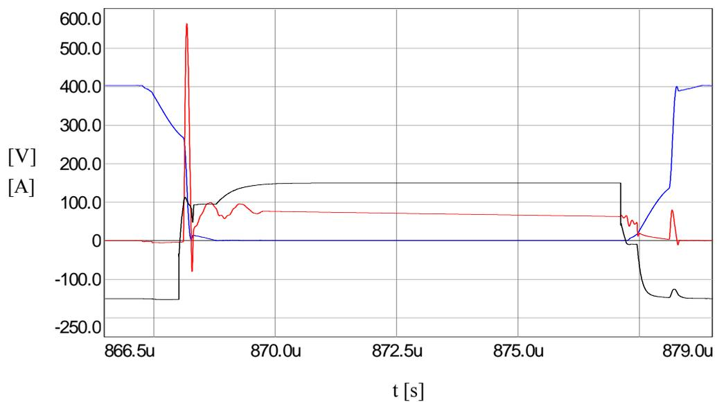
Figure 5.18 Lagging leg IGBT module (T<sub>2</sub>) waveforms at 15% load:
