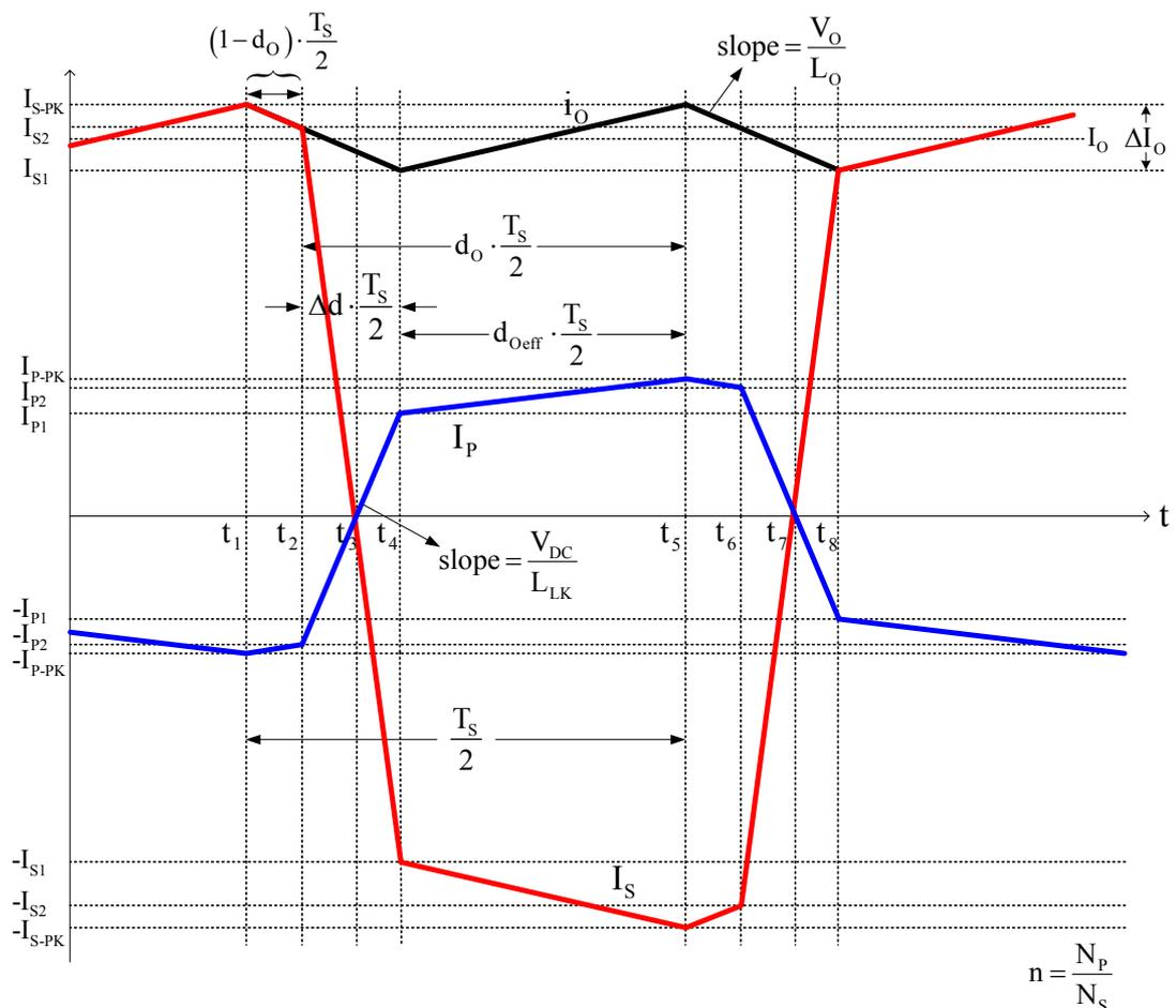
Figure 3.18 The primary, secondary, and load current waveforms.
