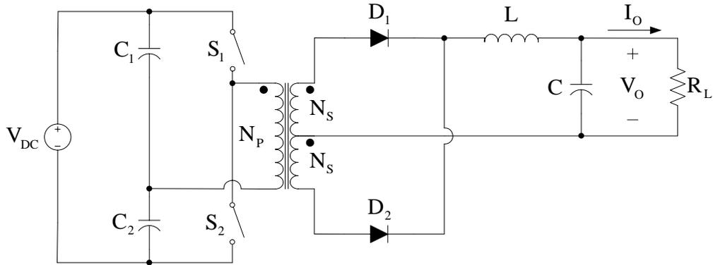
Figure 2.10 The half-bridge DC/DC converter circuit configuration.
