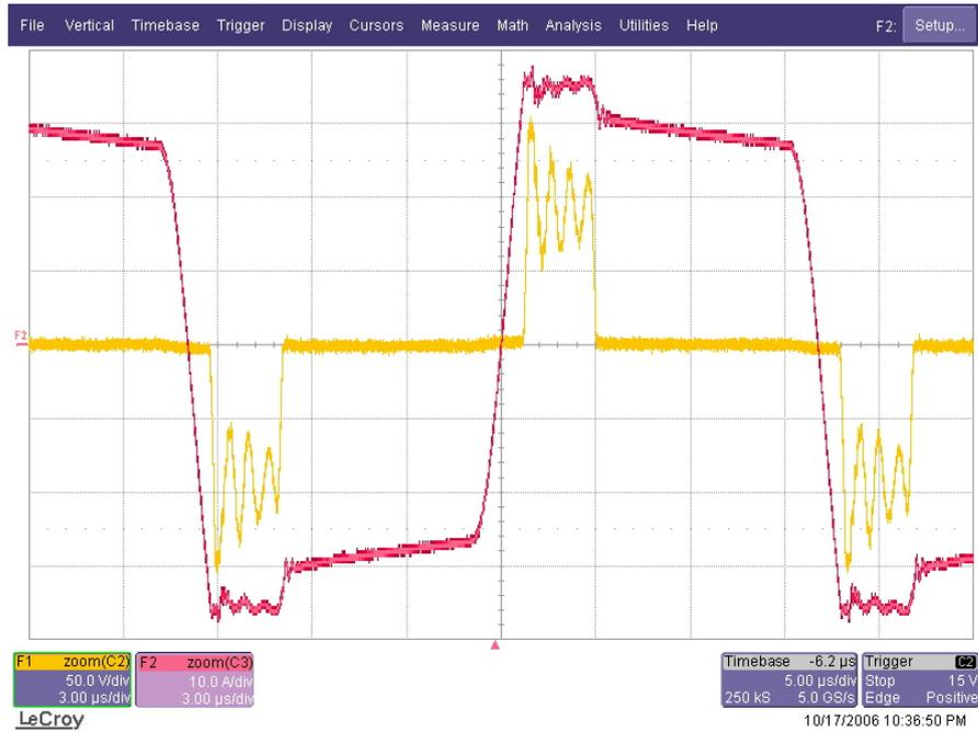
Figure 6.12 Transformer secondary voltage (yellow) and secondary current (red) waveforms at the critical load current (scales: 50 V/div, 10 A/div, 3 μs/div).
