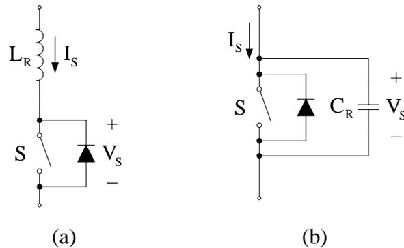
Figure 1.5 The elementary resonant switches for: (a) ZCS, and (b) ZVS operation.
