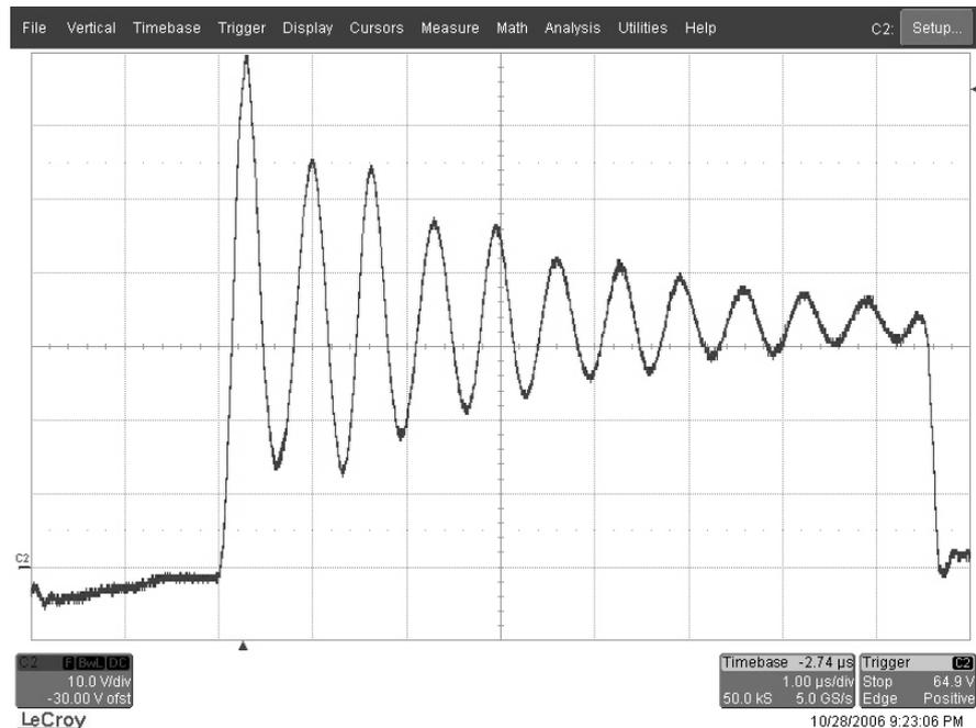
Figure 6.29 The secondary voltage waveform for an input DC voltage of 150 V when no voltage clamp snubber utilized (scales: 10 V/div, 1  $\mu$ s/div).
