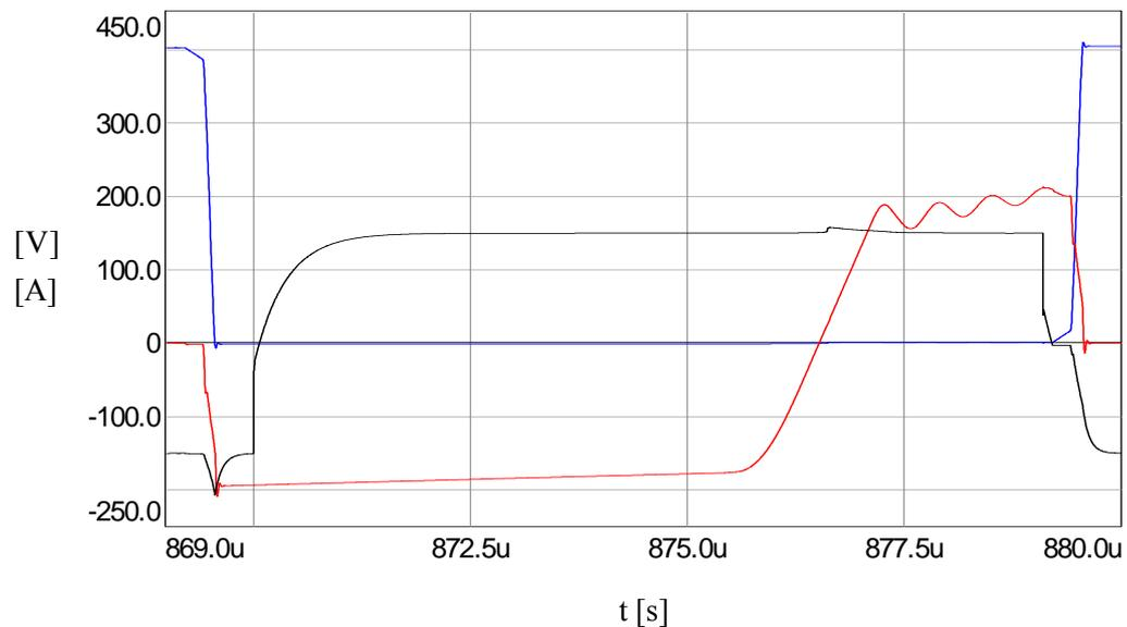
Figure 5.9 Leading leg IGBT module ( $T_4$ ) waveforms at the critical load current:
