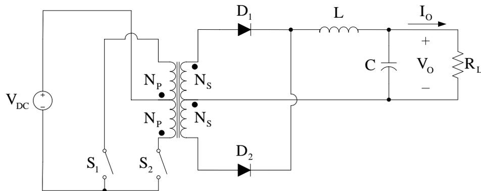
Figure 2.9 The push-pull DC/DC converter circuit configuration.
