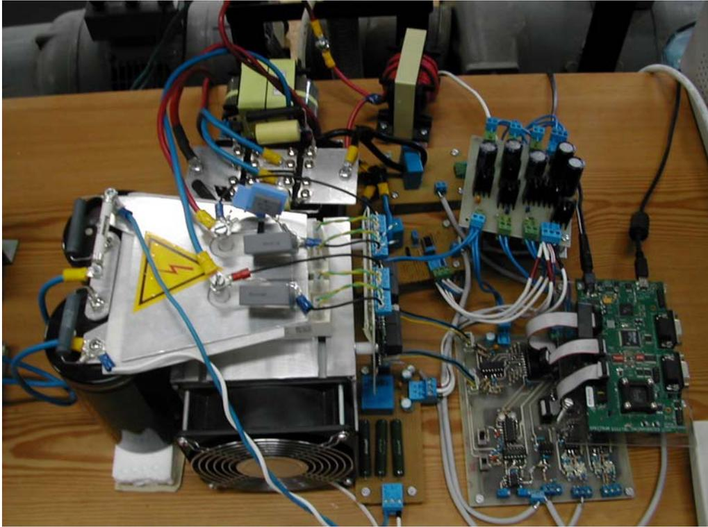
Figure 6.4 Laboratory prototype of the FB-PS-ZVS DC/DC converter.
