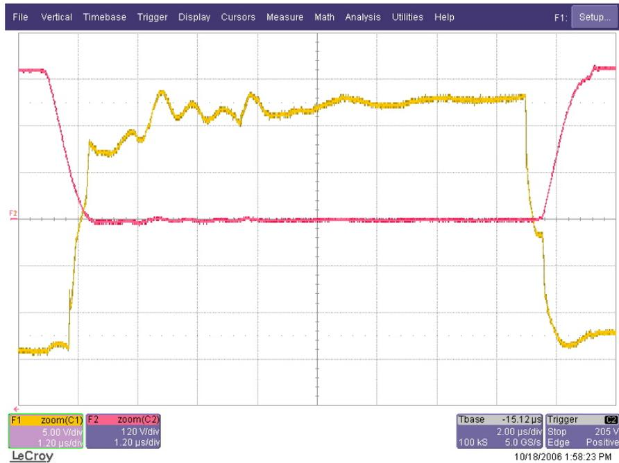
Figure 6.15 Collector-emitter voltage (red) and gate-emitter voltage (yellow) waveforms of the lagging leg IGBT (T<sub>2</sub>) at the critical load current (scales: 120 V/div, 5 V/div, 1.2 μs/div).
