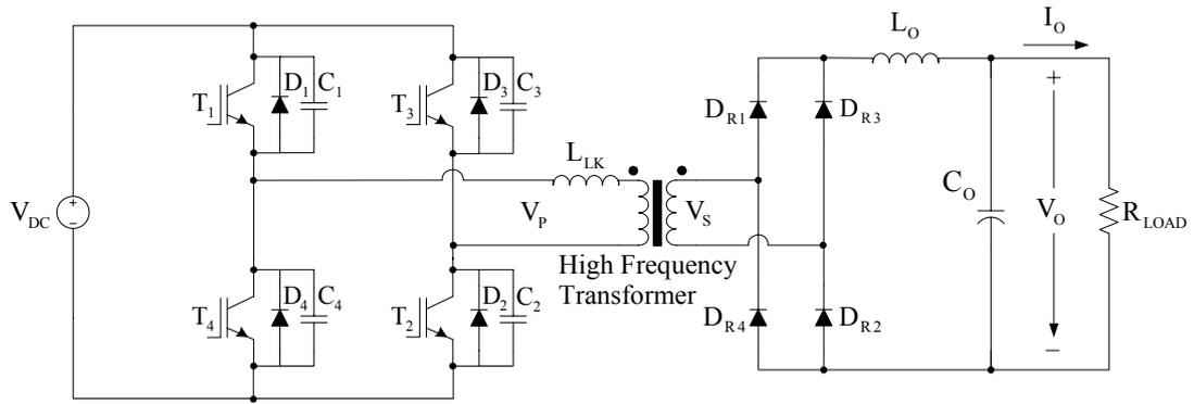
Figure 3.1 The FB-PS-ZVS DC/DC converter circuit diagram.
