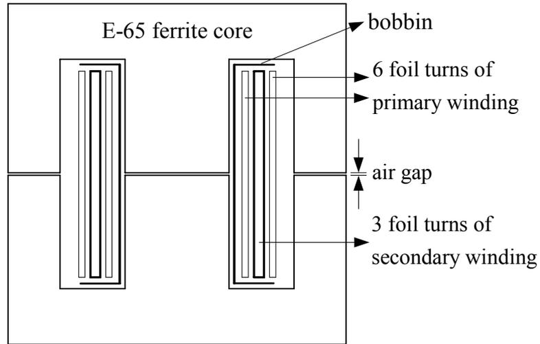
Figure 4.7 The layout of the high frequency transformer.
