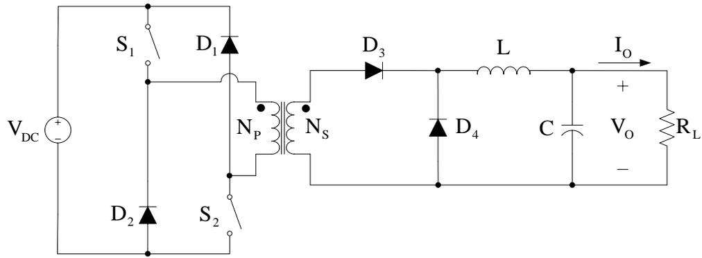
Figure 2.8 The two-switch forward DC/DC converter circuit configuration.
