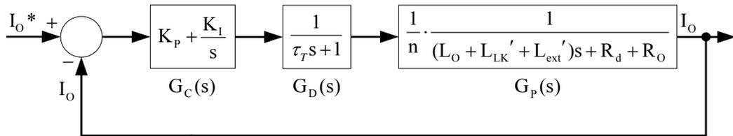
Figure 5.27 The reduced order continuous time model based block diagram of the closed loop current controlled FB-PS-ZVS DC/DC converter system.
