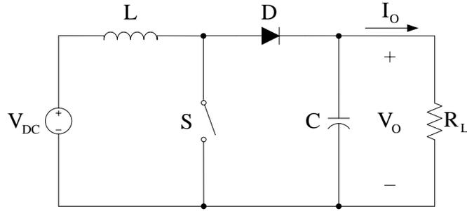
Figure 2.3 The step-up DC/DC converter circuit diagram.
