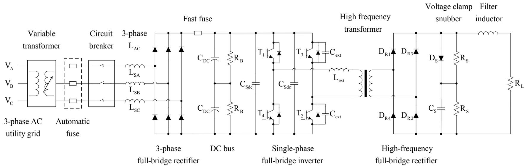
Figure 6.2 The electrical power circuitry of the overall system.
