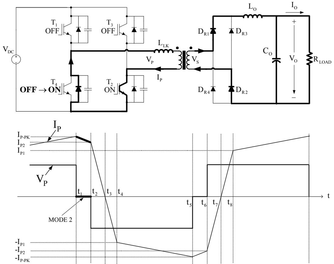
Figure 3.9 The circuit diagram and primary voltage and primary current waveforms of the FB-PS-ZVS DC/DC converter in mode 2.
