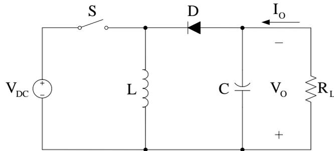
Figure 2.4 The buck-boost DC/DC converter circuit diagram.
