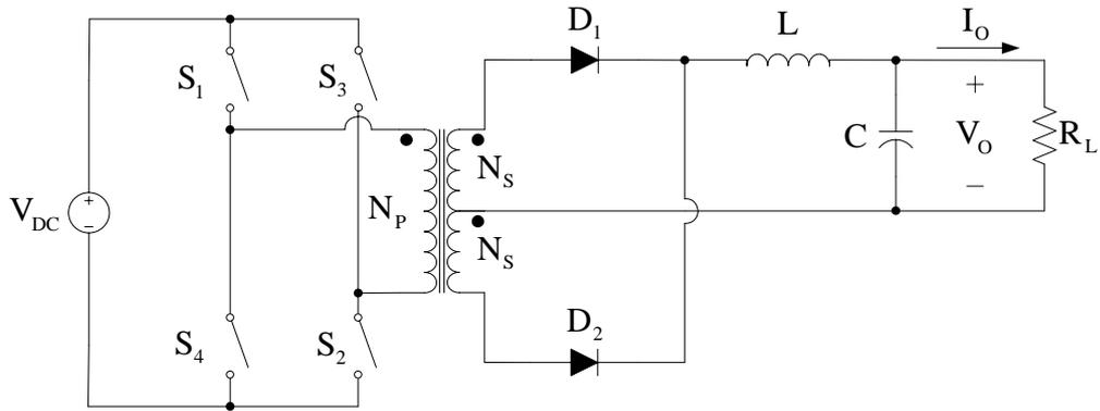
Figure 2.11 The full-bridge DC/DC converter circuit configuration.
