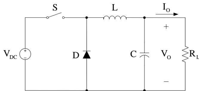
Figure 2.2 The step-down DC/DC converter circuit diagram.
