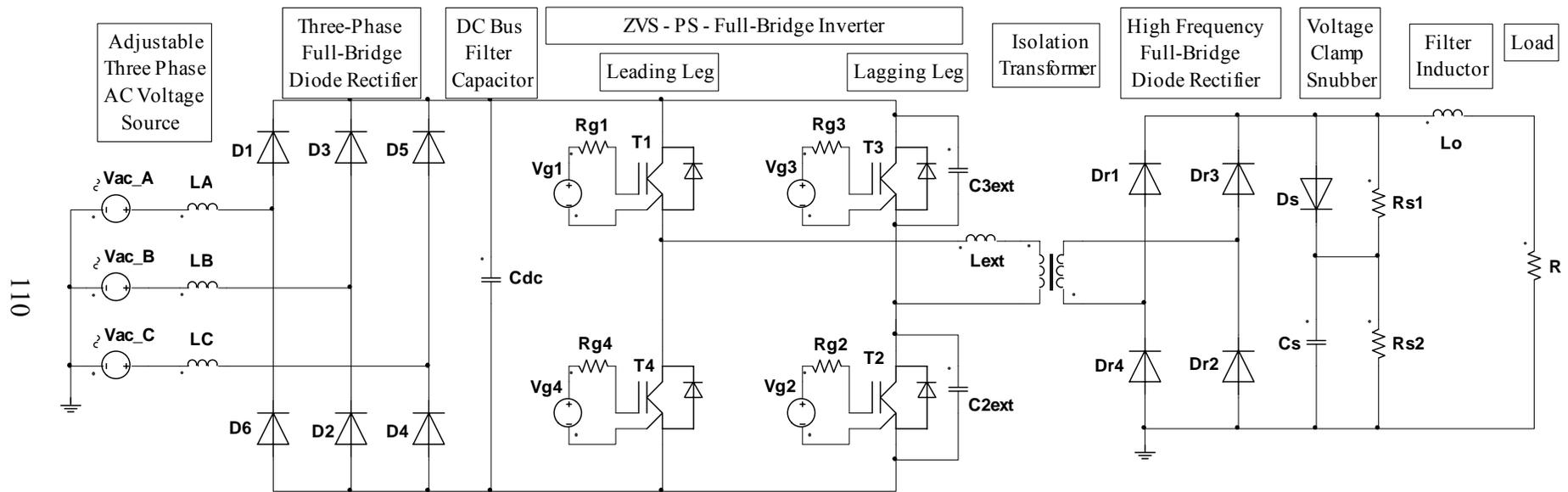
Figure 5.4 Simplorer simulation diagram of the FB-PS-ZVS DC/DC converter system power stage
