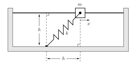
Consider the frictionless mass-spring system shown at rest in the figure. The mass m, connected to the spring with spring constant k, is allowed to slide (horizontally) through the bar, where the displacement from the equilibrium is denoted by x. Obtain the dynamics of this system using the Euler-Lagrange equation.
