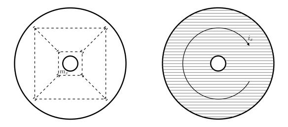
Thanks to this simple observation the question on measuring  $i_x$  we asked earlier can now be rephrased: What instrument does one use to measure the current circulating within a "donut"? The answer is *clamp-on ammeter*. The below figure shows the dual measurements of  $e_x$  and  $i_x$  by a voltmeter and a clamp-on ammeter, respectively. This allows us to conclude that mesh currents are as measurable and hence as real as node voltages.
