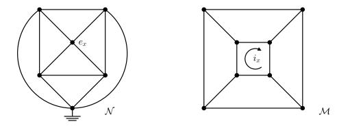
Consider the circuit  $\mathcal{N}$ . Note that " $e_x$  equals the sum of branch voltages associated to any path that connects the node  $n_x$  to the ground node." The dual of this statement for  $\mathcal{M}$  should read: " $i_x$  equals the sum of branch currents associated to any cut that connects the mesh  $m_x$  to the outer mesh." For example, take the path (in  $\mathcal{N}$ ) and its dual cut (in  $\mathcal{M}$ ) shown below. For this particular path-cut pair our dual statements yield
