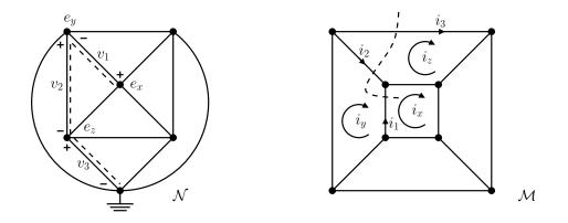
The fact that  $i_x$  is independent of the cut, provided that the cut connects  $m_x$  to the outer mesh, gives  $i_x$  at once a physical character. Namely, the mesh current  $i_x$  is the (well-defined) current circulating in the ring (or "donut") where the inner circle of the ring is contained in the mesh  $m_x$  while the outer circle of
