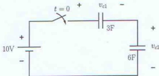
Given  $v_{c1}(0^-) = 3 \text{ V}$ ,  $v_{c2}(0^-) = 1 \text{ V}$ . Find  $v_{c2}(t)$  for  $t > 0$ .
