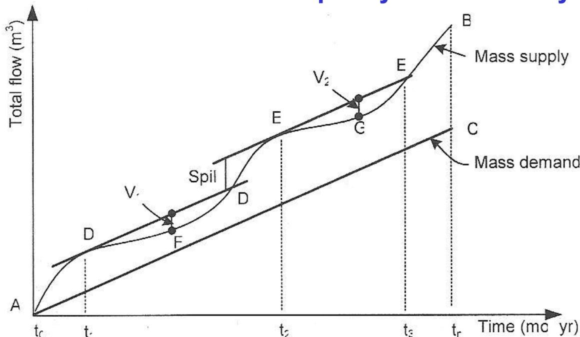
1. The tangents, which are parallel to the demand line, are plotted at the high points (D and E).
