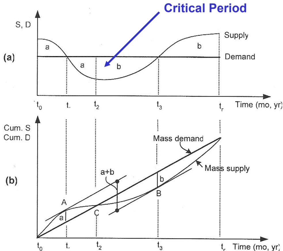
Required storage capacity of the reservoir is the vertical difference  $a+b$
