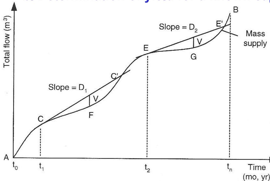
1. The value  $V$  of known reservoir capacity is placed vertically in all the low points in the mass curve and tangents are drawn to the previous high points.
