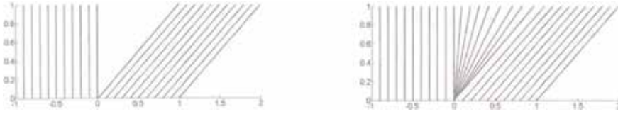
Figure 5. For initial value u_L < u_R , characteristic solutions u_1(t, x) and u_2(x, t) with rarefaction fan.
