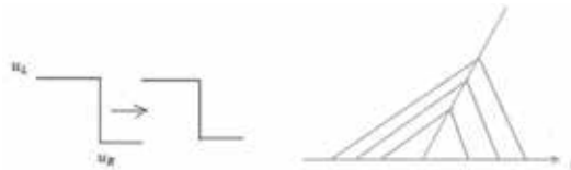
Figure 1. For the initial value u_L > u_R , characteristics, and shock wave.
